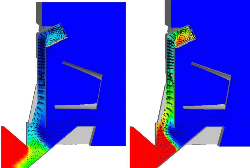
**Figure 8:** Fume distribution and velocity vectors 0.5m from the ladle centre-line for new hood design at the low flow rate case, for two fume generation cases 360 Nm<sup>3</sup>/hr (left) and 1440 Nm<sup>3</sup>/hr (right).
