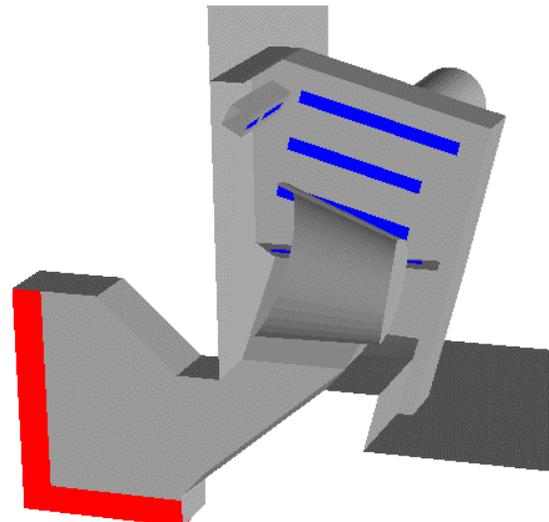
**Figure 2:** Three-dimensional CFD model of the original charge port design cut through the centre-line, blue areas indicate slots and the red area is the fume entry boundary condition in the furnace.
