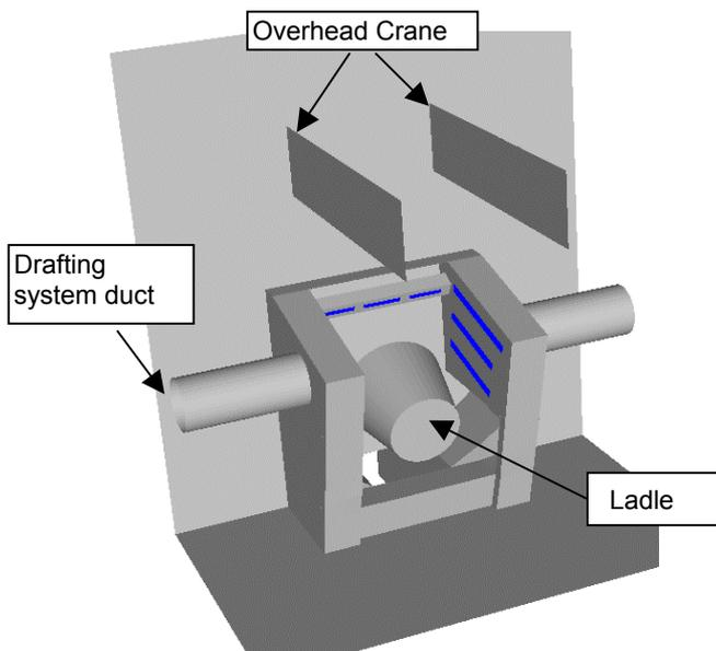
**Figure 1:** Three-dimensional CFD model geometry of the original charge port, drafting slots shown in blue.
