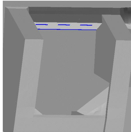
**Figure 5:** Three-dimensional geometry of the new charge port design without the ladle (drafting slots shown in blue)
