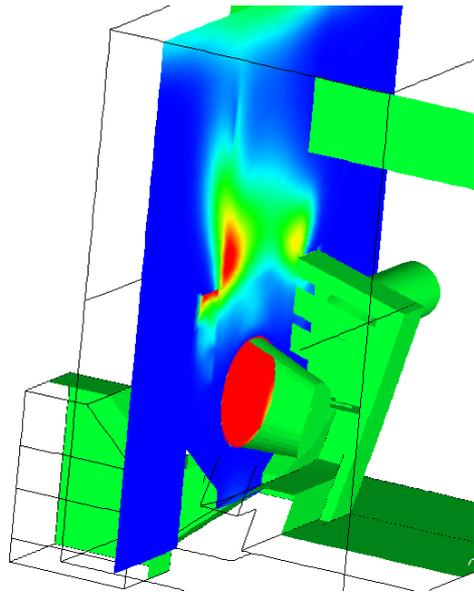
**Figure 4:** Fume distribution for the original design at the low flow rate case on a plane near the ladle opening.
