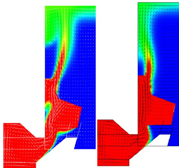
**Figure 3:** Side view of fume distribution for the original design at the low (left) and high (right) flow rate on a central plane.
