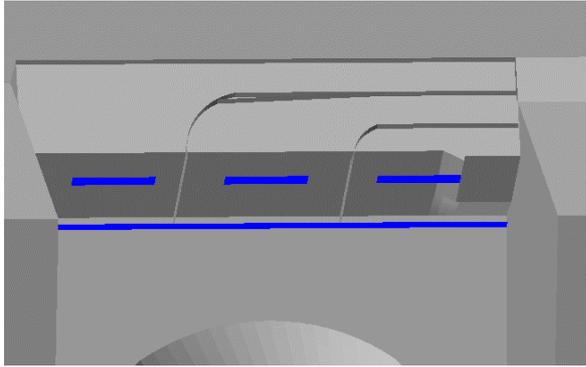
**Figure 7:** Detail of the slots and baffling in the top part of the new hood with the outer faces removed (blue regions are the slots)
