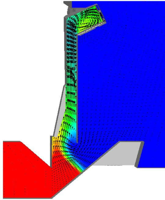
**Figure 9:** Fume distribution and velocity vectors 0.5m from the ladle centre-line for new hood design without the ladle at the medium flow rate case with high fume generation.
