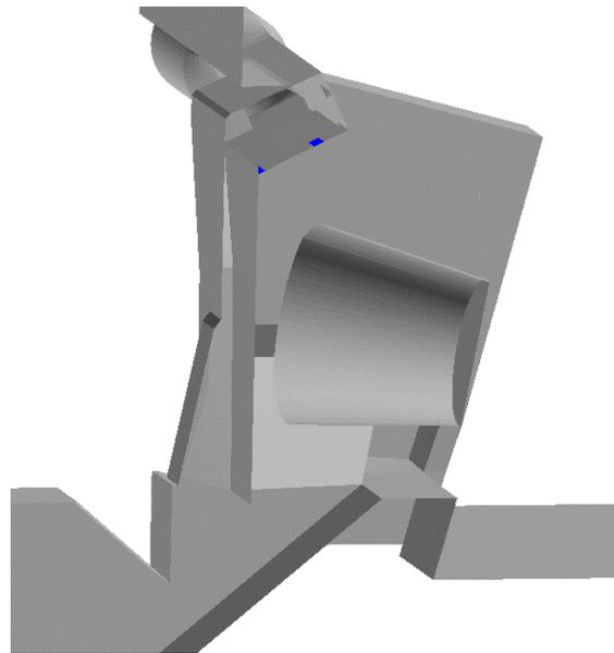
**Figure 6:** Three-dimensional geometry of the new charge port cut through centre line.
