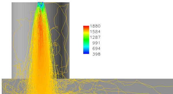
**Figure 5:** Particle Trajectories and Temperature
