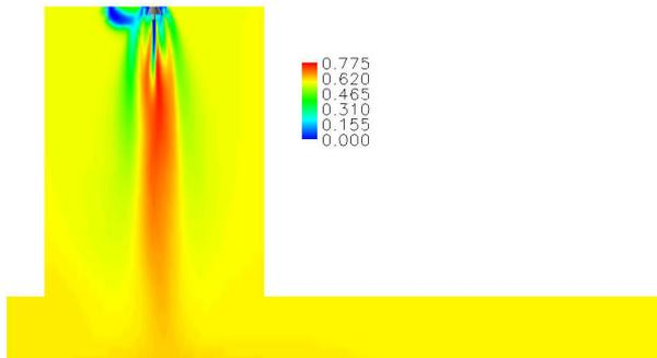
**Figure 4:** SO<sub>2</sub> Content in Flash Furnace
