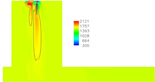
Figure 2: Temperature in Flash Smelting Furnace
