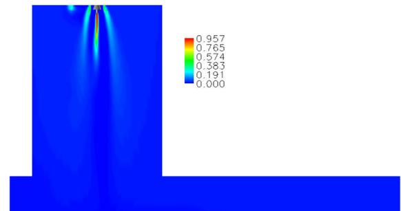
Figure 3: O<sub>2</sub> Content in Flash Furnace
