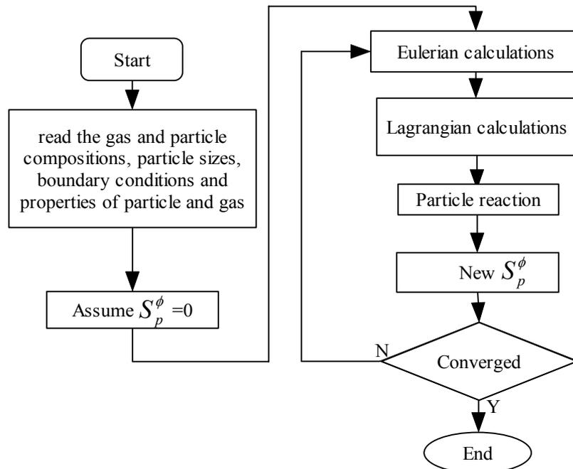
Figure 1: Overall solution algorithm of the mathematical model
