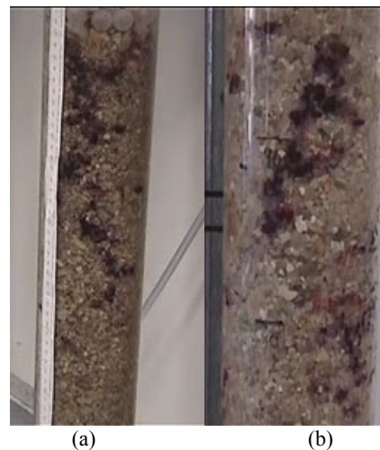
Figure 1: (a) Liquid flow distribution in the column containing 9.5 mm grade quartz when column is under operation. (b) close-up of the 1 m column
