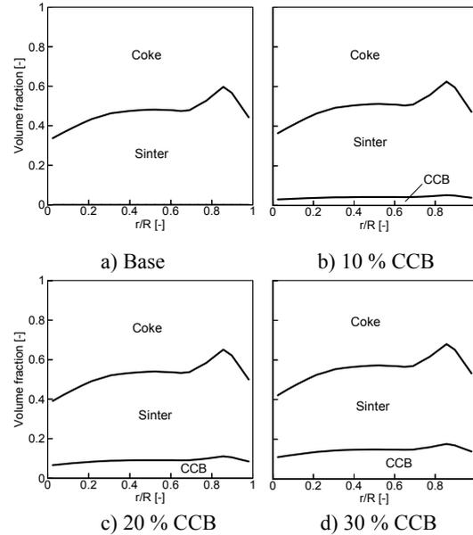
**Figure 1:** Charging patterns of solid components used in this study.
