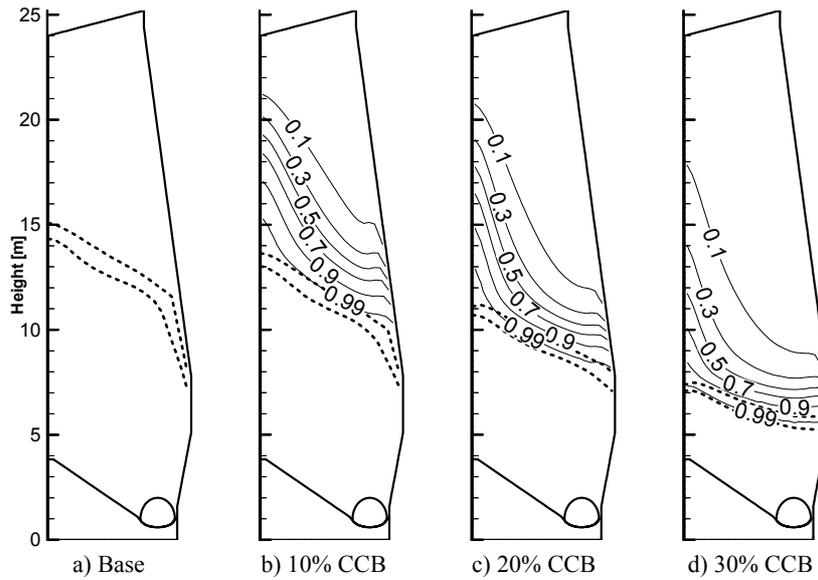
Figure 4: Effect of CCB charging ratio on distribution of CCB reduction degree [unit: -].
