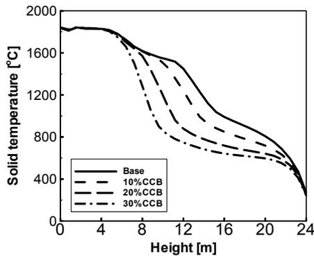
Figure 3: Distribution of averaged solid temperature along furnace height.
