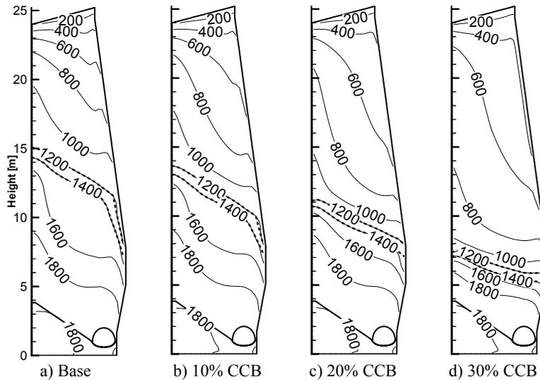
Figure 2: Effect of CCB charging ratio on distribution of solid temperature [unit: °C].
