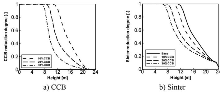
Figure 5: Distribution of averaged reduction degree along furnace height.
