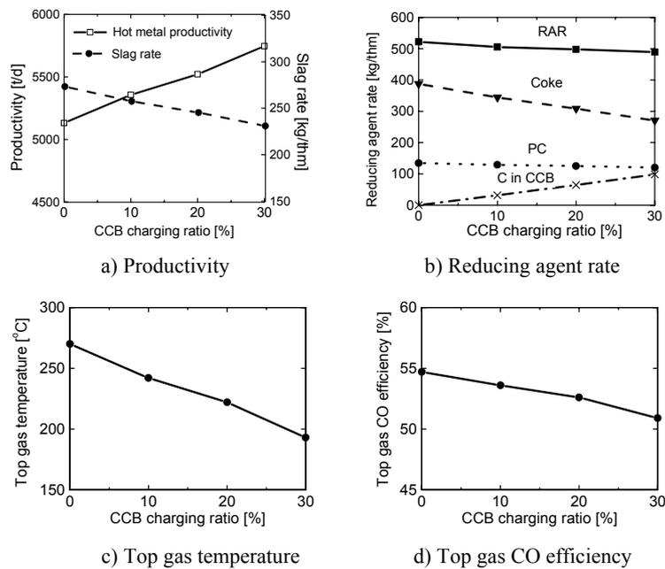
Figure 6: Predicted operational parameters under different charging rate of CCB.
