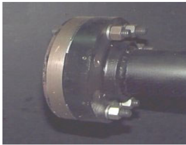
Figure 1: Photograph showing the experimental set-up of the pipe, flange and blank end.
