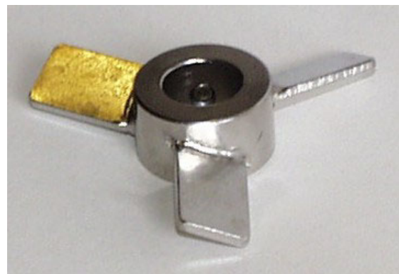
Figure 7: The impeller studied (3PBT30; D=48mm)
