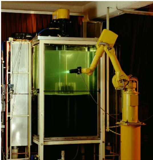
**Figure 2:** Research vessel shown with LDV head manipulated by robot arm for fluid velocity measurement.
