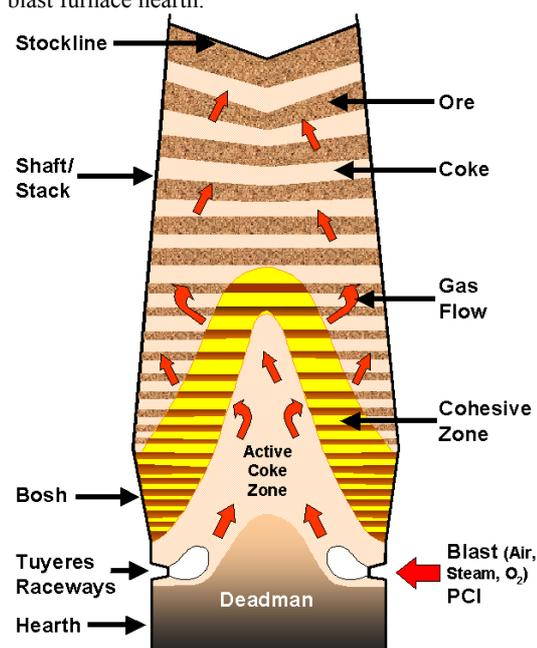
**Figure 1:** The blast furnace process.
