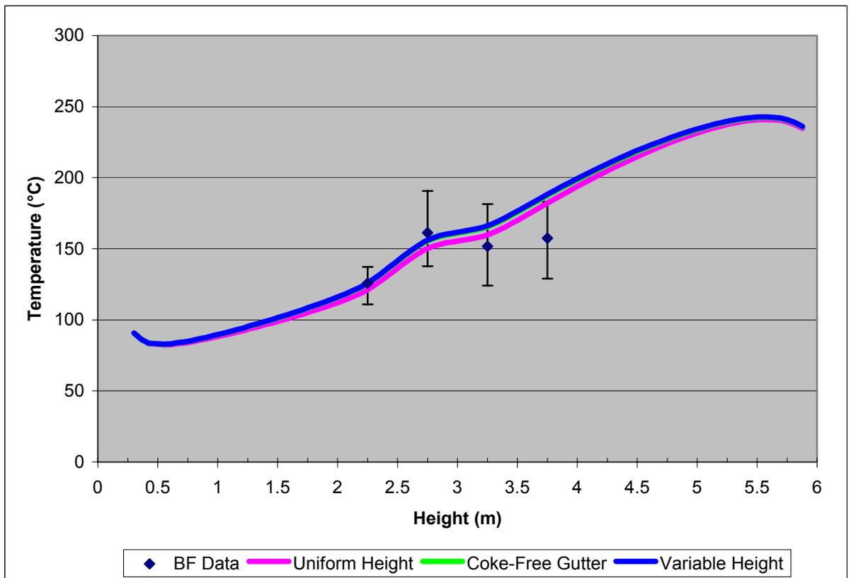
Figure 7: Comparison of sidewall thermocouple with predictions of CFRM for different CFL shapes.
