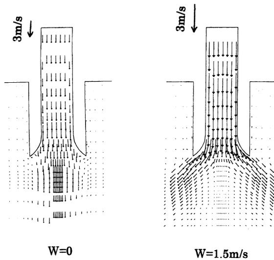
**Figure 4:** Velocity distributions at the nozzle-outlet in the cases with and without swirl.  $V_z$  is 1.5 m/s in the immersion nozzle.
