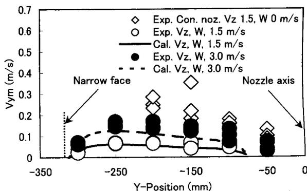
**Figure 7:** Velocity of the surface flow at 11 mm below the meniscus.
