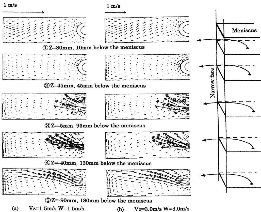
**Figure 5:** Flow patterns with swirl at various depths below the meniscus, 12, 48, 148 and 198 mm for the water model in the cases;  $V_z$  in nozzle, 1.5 m/s and 3 m/s; entrance tangential velocity  $W$ , 1.5m/s and 3 m/s
