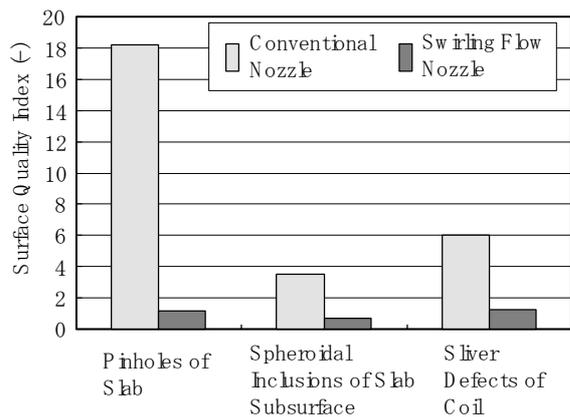
**Figure 9:** Effect of swirling flow immersion nozzle on surface quality of slabs and coils.
