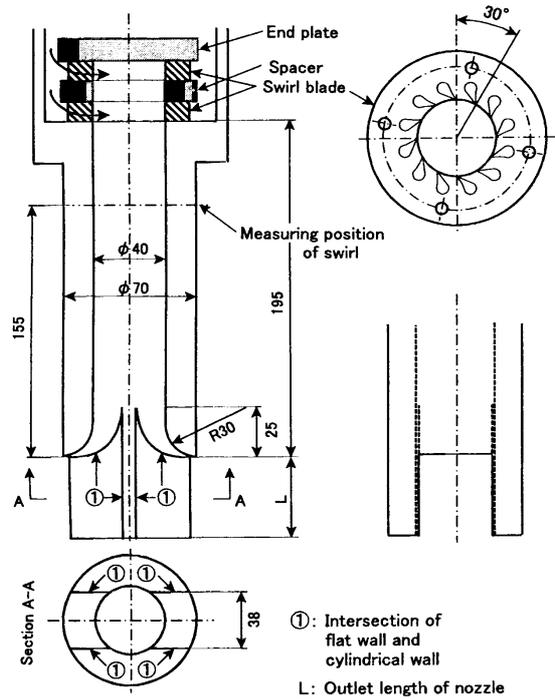
**Figure 2:** Schematic diagram of bottomless nozzle with swirl blade.
