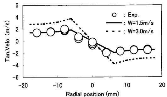
**Figure 3:** Radial profile of the tangential velocity,  $W$ , at the entrance of the nozzle.
