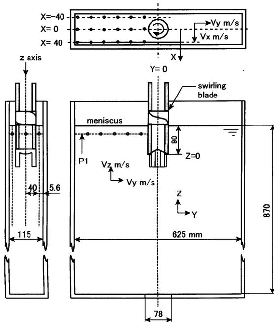
**Figure 1:** Schematic diagram of model mold, showing swirl blade and positions for measuring velocity.
