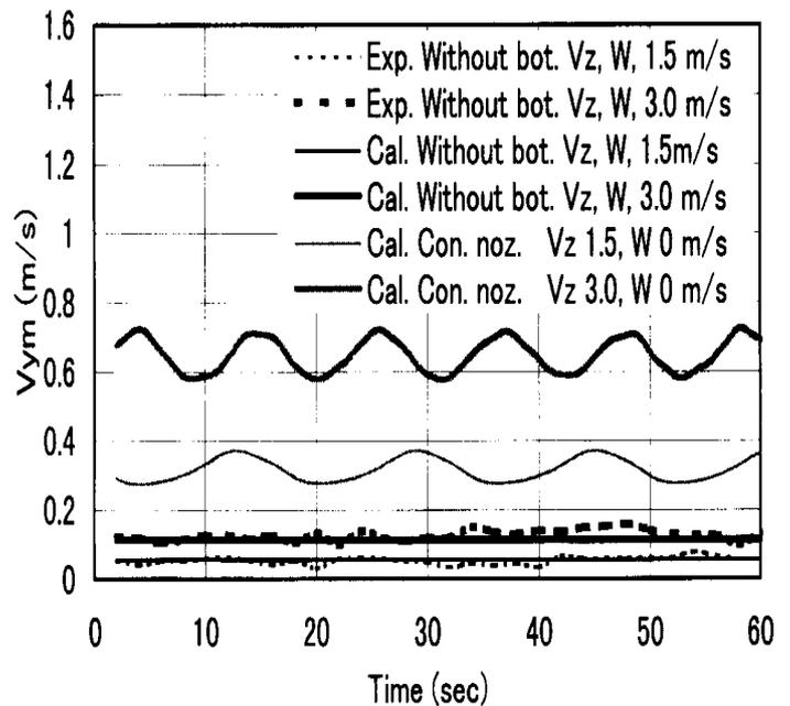
**Figure 8:** Calculated velocity fluctuation of the surface flow at 11 mm below the surface ( $Y = -150$  mm at the center line section).
