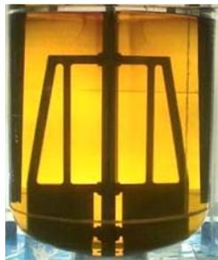
Figure 2: Maxblend impeller
