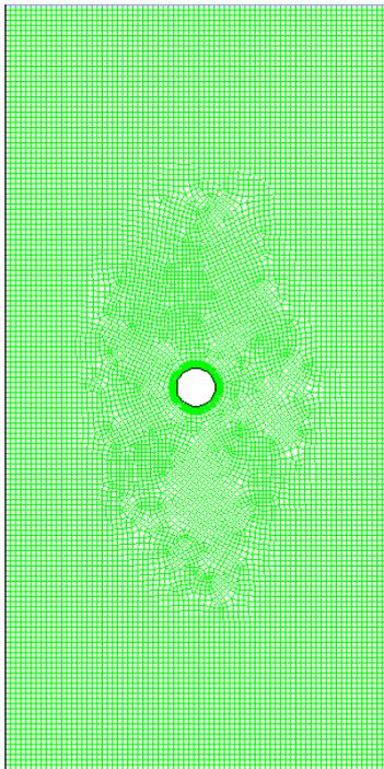
**Figure 3:** Schematic diagram of geometry for bubble of 1.5 mm diameter with unstructured mesh.
