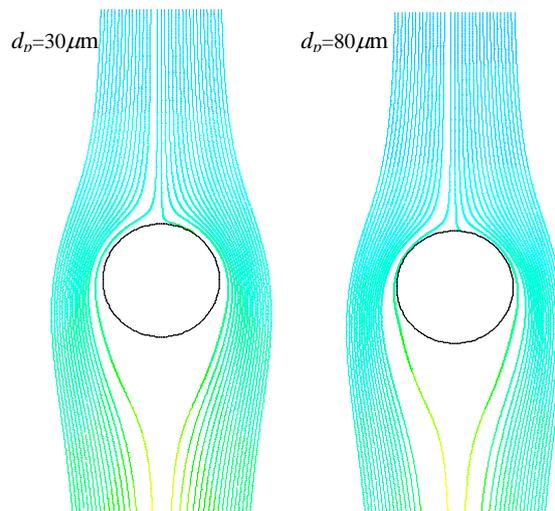
**Figure 10:** Tracks of particle streamlines around 1.0 mm diameter bubble with structured mesh.
