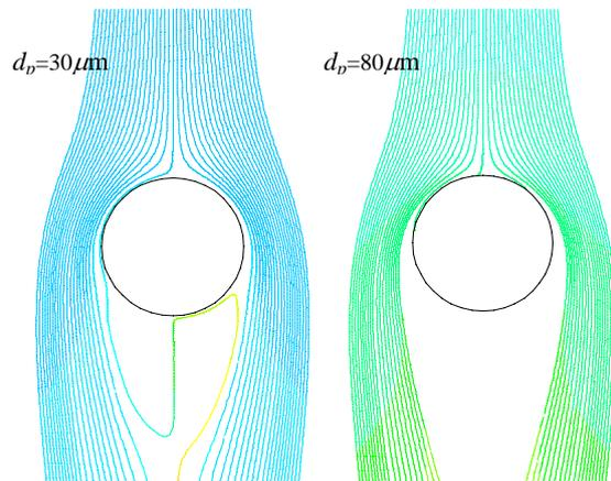
**Figure 9:** Tracks of particle streamlines around 1.5 mm diameter bubble with unstructured mesh.
