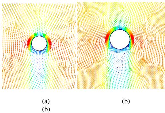
**Figure 6:** Velocity vectors around bubbles with unstructured mesh (a) 1.0 mm dia.; (b) 1.5 mm dia.
