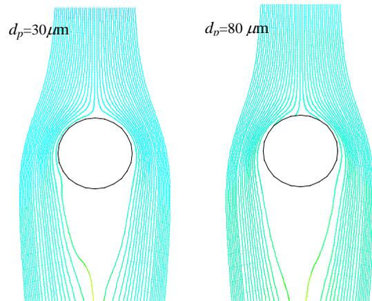
**Figure 8:** Tracks of particle streamlines around 1.0 mm diameter bubble with unstructured mesh.
