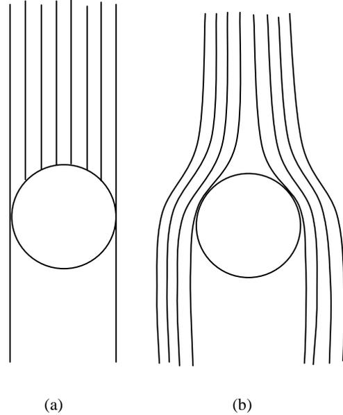
**Figure 1:** Schematic diagram for collision probability; (a) bubbles having probability of collision; (b) bubbles that actually collide
