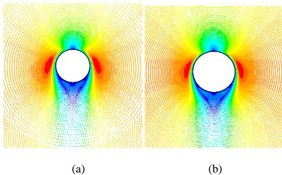
**Figure 7:** Velocity vectors around bubbles with structured mesh (a) 1.0 mm dia.; (b) 1.5 mm dia.
