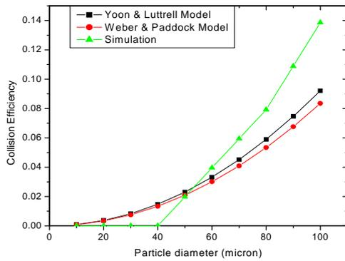
**Figure 12:** Comparison of the results of CFD simulations and hydrodynamic models for 1.0 mm bubble with unstructured mesh geometry.
