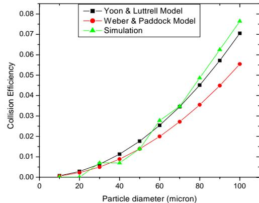
**Figure 15:** Comparison of the results of CFD simulations and hydrodynamic models for 1.5 mm bubble with structured mesh geometry.
