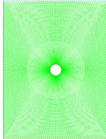
**Figure 4:** Schematic diagram of geometry for bubble of 1.0 mm diameter with structured mesh.
