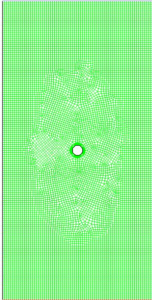
**Figure 2:** Schematic diagram of geometry for bubble of 1.0mm diameter with unstructured mesh.
