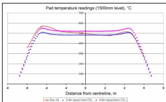
**Figure 13:** Comparison of pad thermocouple with model predictions for 400 mm and 800 mm raised hemispherical shaped coke free layer (see Figs 9-10)
