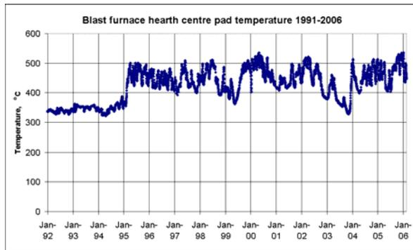
**Figure 6:** Campaign centre pad temperature data for PKBF5
