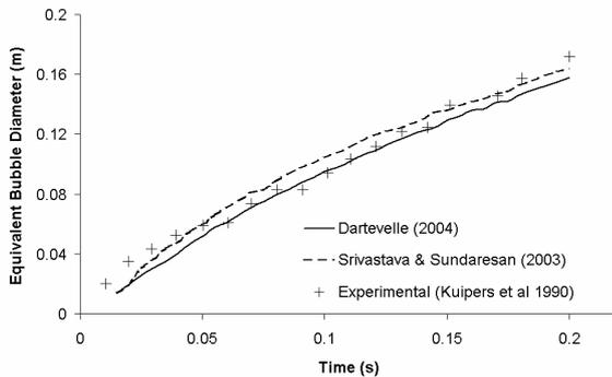
**Figure 1:** Comparison of equivalent bubble diameter.
