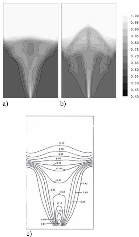
**Figure 3:** Time averaged (over 2 seconds) porosity contour plots of the a) Dartevelle model, b) Srivastava & Sundaresan model and c) experimental contours of Kuipers et al 1990.
