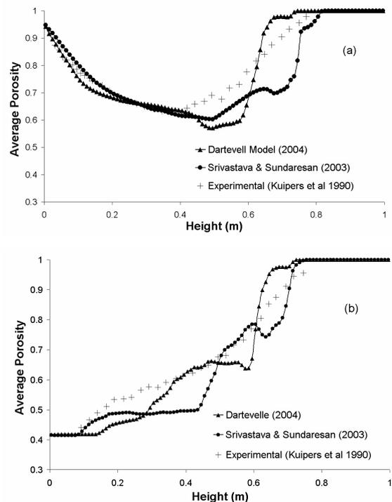
**Figure 2:** Average porosity profiles along the height of the bed at (a)x= 0.375cm and (b) x= 9.375cm from the central jet.
