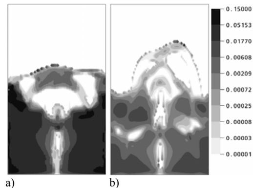
**Figure 4:** Comparison of average solids viscosities at 3.5 seconds; of the a) Dartevelle model and b) Srivastava and Sundaresan model.
