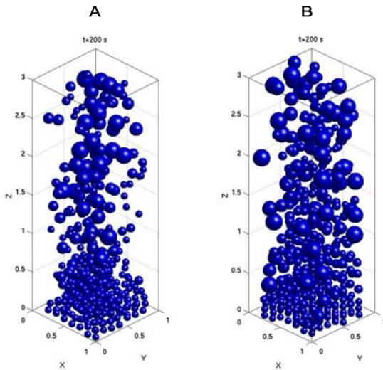
**Figure 5:** Influence of bubble-bubble interactions on snapshots of the bubbles after 200 s: A) without bubble-bubble interactions; B) with bubble-bubble interactions (Farrokhalae, 1979).
