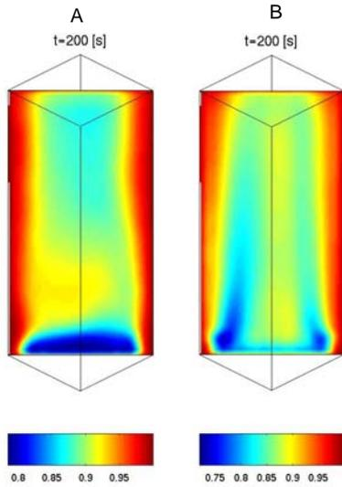
**Figure 4:** Influence of bubble-bubble interactions on the time-averaged porosity plots: A) without bubble-bubble interactions; B) with bubble-bubble interactions (Farrokhalae, 1979).
