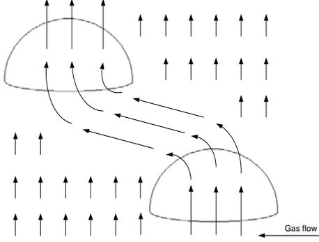
**Figure 1:** Schematic representation of the gas flow through a freely bubbling fluidised bed consisting of Geldart B type solids.
