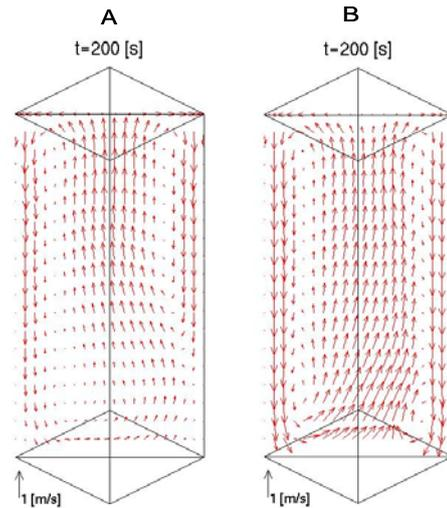
**Figure 3:** Influence of bubble-bubble interactions on the time-averaged emulsion phase velocity profiles: A) without bubble-bubble interactions; B) with bubble-bubble interactions (Farrokhlaee, 1979).
