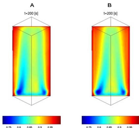
**Figure 8:** Time-averaged porosity plot. The case with the small bubble diameter is A) and the case with large maximum bubble diameter is B).
