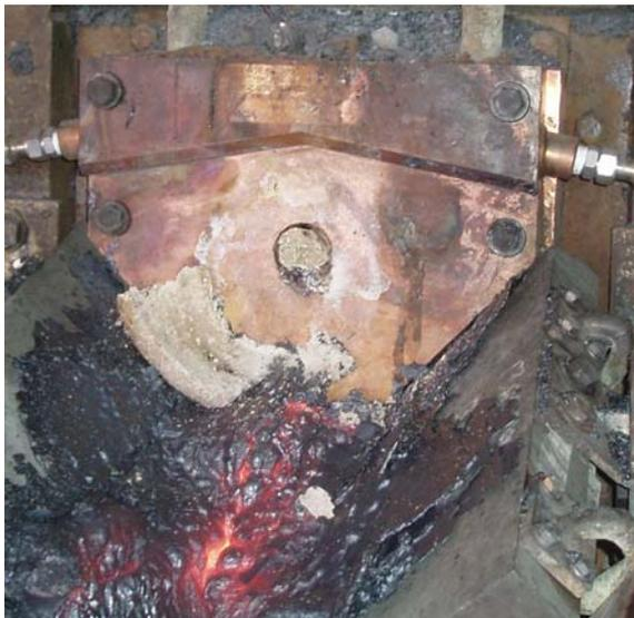
**Figure 7:** Bateman Design Breast Plate Immediately after Plugging
