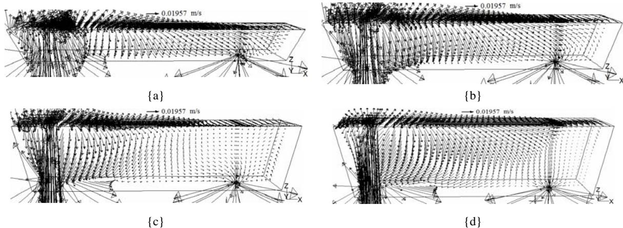
**Figure 5:** Velocity vectors at a vertical plane passing through the inlet and outlet as well as on the top free surface for different bath heights of the tundish. (a) 120 mm (b) 180 mm (c) 260 mm (d) 320 mm
