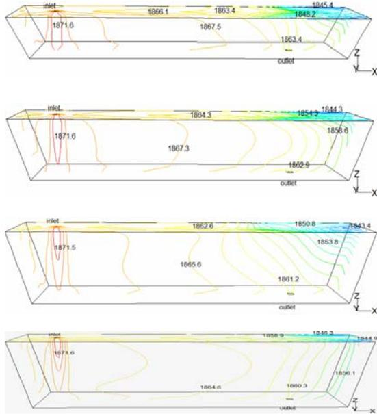
**Figure 6:** Temperature contours for different cases of bath heights (as in figure 5)
