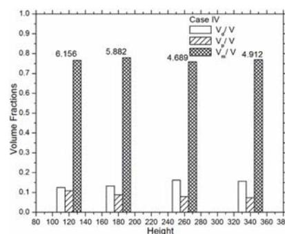
**Figure 4:** (a) RTD curves for different bath height of tundish and (b) Volume fractions for different bath height of tundish, Case {a, b, c, d}
