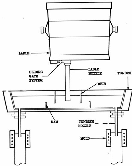
**Figure 1:** Schematic of a continuous casting process
