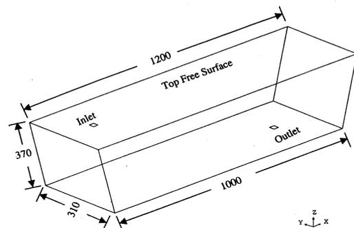
**Figure 2:** Geometry of the tundish [Singh and Koria (1993)] (Dim. in mm.)
