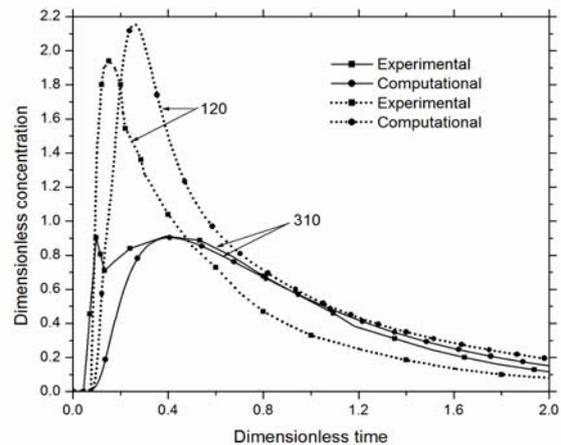
**Figure 3:** Comparison of computational RTD curve for two tundishes with experimental observations of Singh and Koria
