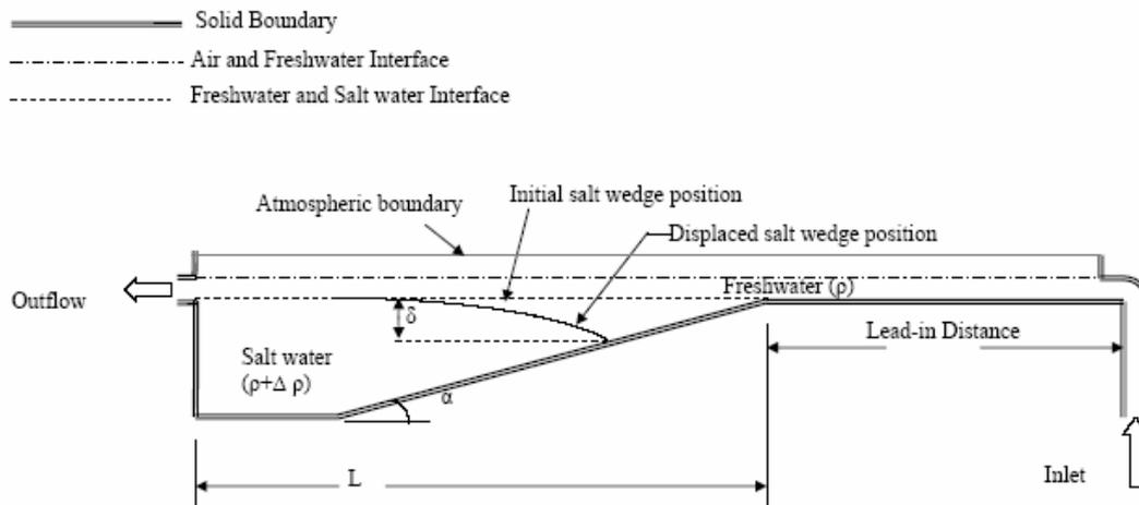
**Figure 4:** Schematic diagram of the physical model for numerical study (not to scale)
