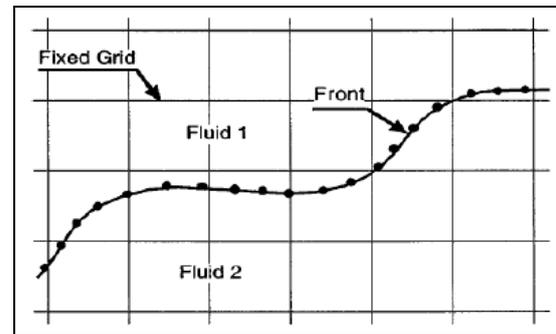
**Figure 1:** The governing equations are solved on a fixed grid but the phase boundary is represented by a moving "front," consisting of connected marker points.
