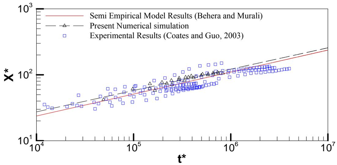
**Figure 5:** Comparison of semi empirical, numerical and experimental (Coates and Guo, 2003) results for non-dimensional wedge displacement ( $x^*$ ) with respect to non-dimensional time ( $t^*$ ).
