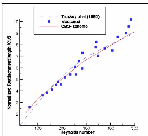
**Figure 2b.** Comparison of the size of recirculation zone for an expansion ratio of 2.37.
