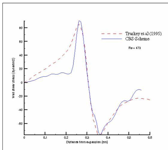
**Figure 2c.** Distribution of wall shear stress along the recirculation zone for  $Re=473$  with an expansion ratio of 2.37.
