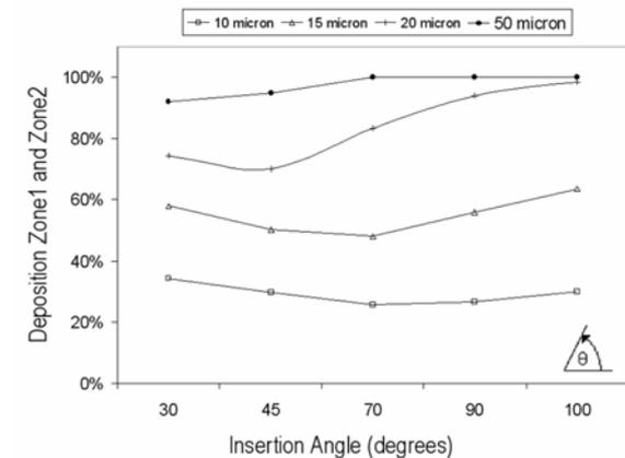
**Figure 5:** Deposition in zone1 and zone2 for monodispersed particles released uniformly from the inlet surface at 10m/s for different insertion angles.
