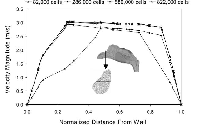
**Figure 1:** Velocity profiles at the nasal valve region for different nasal cavity models showing grid independence at 586000 cells.
