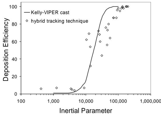
**Figure 2:** Deposition efficiency for monodisperse particles released passively from the nostril inlet subjected to airflow rates of 20L/min, 30L/min and 40L/min using a hybrid tracking technique.
