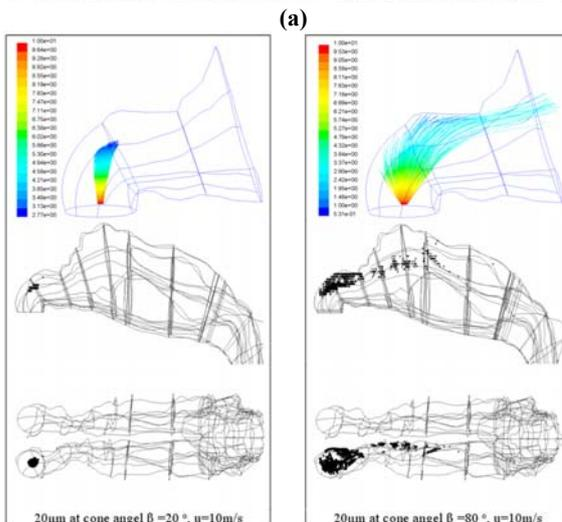
**Figure 8:** Particle trajectories coloured by velocity magnitudes (m/s) and local deposition sites for mono-sized particles released at 10m/s from a small internal diameter at the centre of the nostril inlet surface. The spray cone angles ranged from 20° and 80°. (a) 15 $\mu\text{m}$  particles and (b) 20 $\mu\text{m}$  particles released
