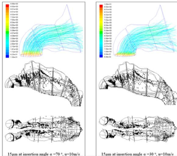
**Figure 6:** Particle trajectories coloured by velocity magnitudes (m/s) and local deposition sites for 15 $\mu\text{m}$  particles released uniformly from the inlet surface at insertion angles 70° and 30°.
