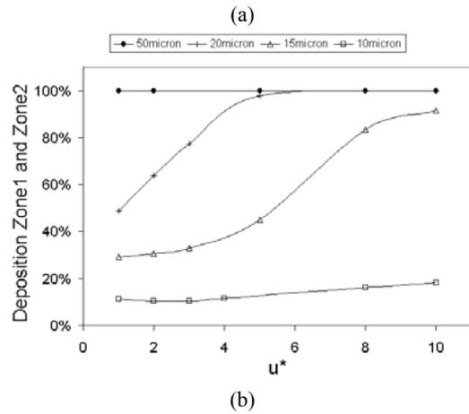
**Figure 3:** a) Segmented view of the front region of the nasal cavity showing Zone 1, 2 and 3. b) Total deposition efficiency in Zone 1 and Zone 2 of the nasal cavity for different particle injection velocity  $u^*$ , where  $u^* = u_{pi} / u_g$
