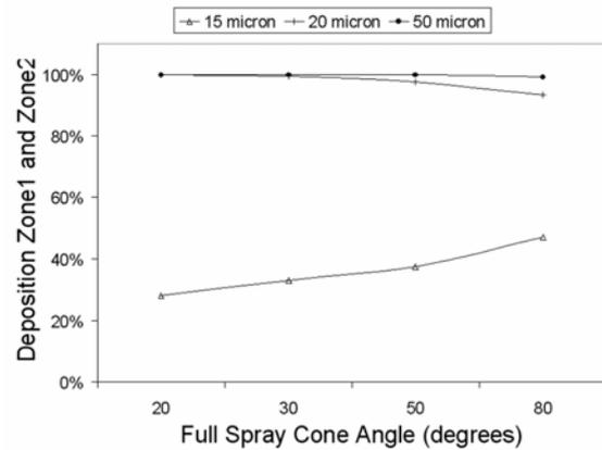
**Figure 7:** Total deposition in zone1 and zone2 for monodispersed particles released at 10m/s from a small internal diameter at the centre of the nostril inlet surface. The spray cone angles ranged from 20° and 80°.
