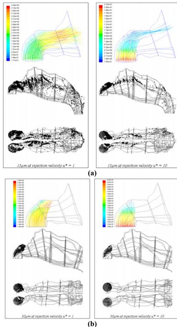
**Figure 4:** Particle trajectories coloured by velocity magnitudes (m/s) and local deposition sites for mono-sized particles released uniformly from the inlet surface normal to the nostril openings at  $u^*=1$  and  $u^*=10$ . (a) 15µm particles and (b) 50µm particles.
