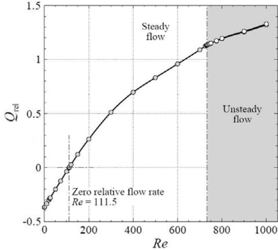
**Figure 6:** Flow rate relative to spheres ( $Q_{rel}$ ) plotted against Reynolds number for a geometric configuration with  $SR = 1.0$  and  $DR = 0.6$ . Unsteady flow was detected in the shaded region, and in this region lines through local minima and maxima in the time-varying flow rate is plotted.
