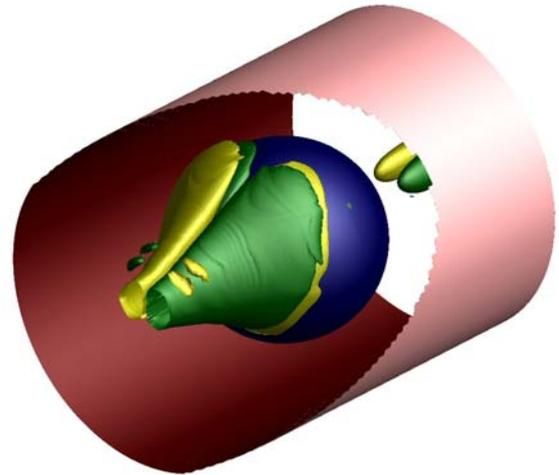
**Figure 10:** Iso-surface plot showing the structure of the non-axisymmetric flow at  $Re = 360$  with  $DR = 0.6$  and  $SR = 1.0$ , computed using the three-dimensional solver and mesh. Flow is from top right to bottom left, yellow and green contours reveal negative and positive regions of streamwise vorticity, respectively. The sphere is coloured blue, and a cutaway of the tube is provided to reveal the relevant isosurfaces.
