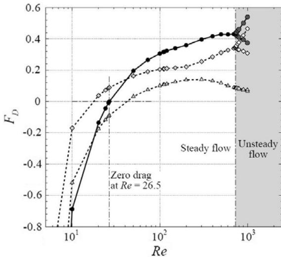
**Figure 7:** Total drag force (solid lines and “•”) and pressure and viscous (dotted lines and “◊” and “Δ”, respectively) contributions plotted against Reynolds number for a geometric configuration with  $SR = 1.0$  and  $DR = 0.6$ . Unsteady flow was detected in the shaded region, and in this region lines through local minima and maxima in the drag forces are plotted.  $F_D$  acts in the axial direction.
