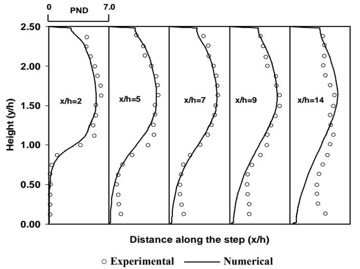
Fig.11 Particle number density for 70µm copper particles
