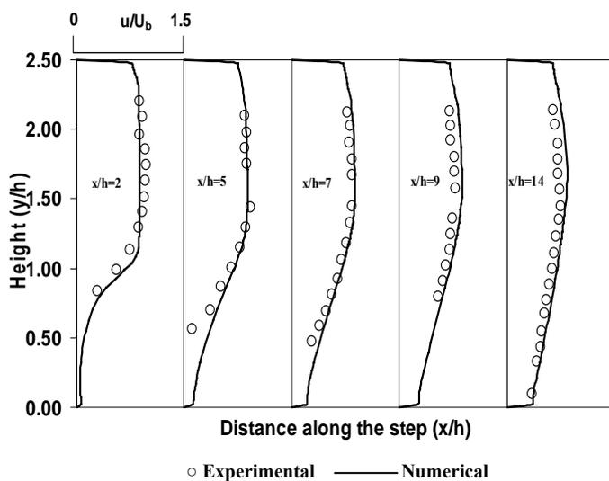
Fig.5 Streamwise mean velocity for 150µm glass particles
