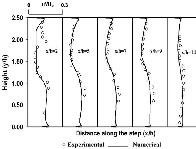
Fig.8 Fluctuating streamwise particle velocities for 70µm copper particles
