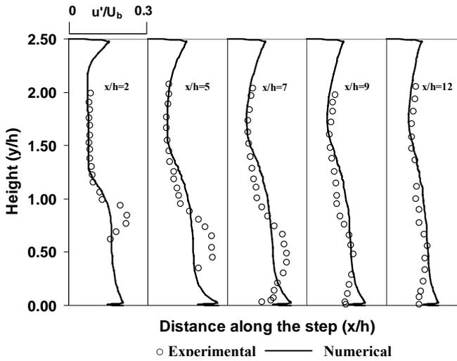
Fig.7 Fluctuating streamwise particle velocities for 90µm glass particles
