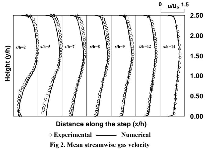
**Fig 2.** Mean streamwise gas velocity
