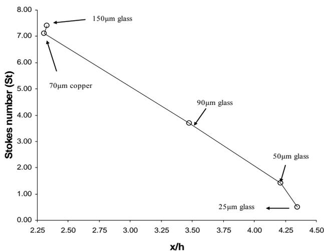
Fig.12 Re-attachment point Vs Stokes number
