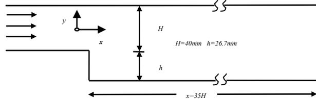
**Fig.1** Backward facing step geometry
