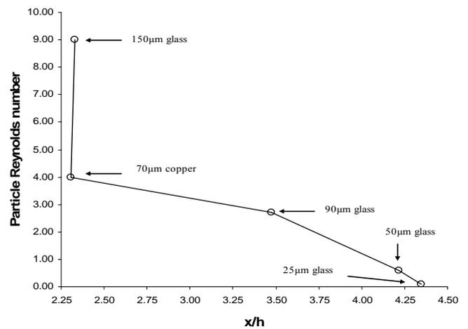
Fig.13 Re-attachment point Vs particle Reynolds number
