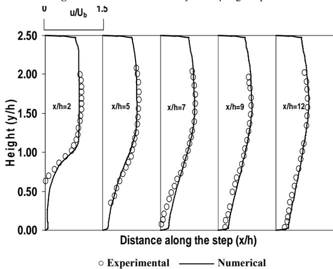
Fig.4 Streamwise mean velocity for 70µm copper particles
