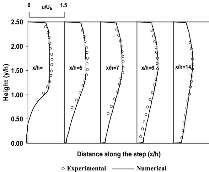
Fig.3 Streamwise mean velocity for 90µm glass particles
