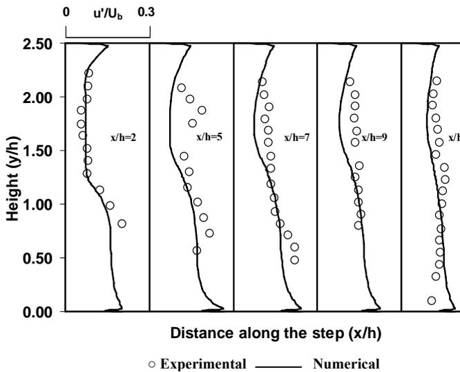
Fig. 9 Fluctuating streamwise particle velocities for 150µm glass particles
