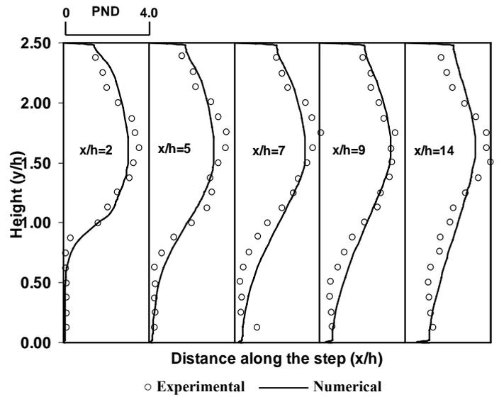
Fig.10 Particle number density for 90µm glass particle
