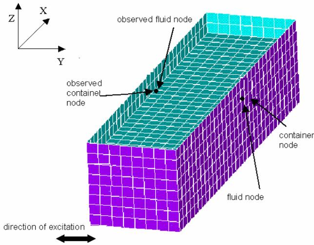
**Figure 1.** The numerical model and the location of the observed nodes. The container has the dimensions of 1.6 m x 0.4 m x 0.4 m.
