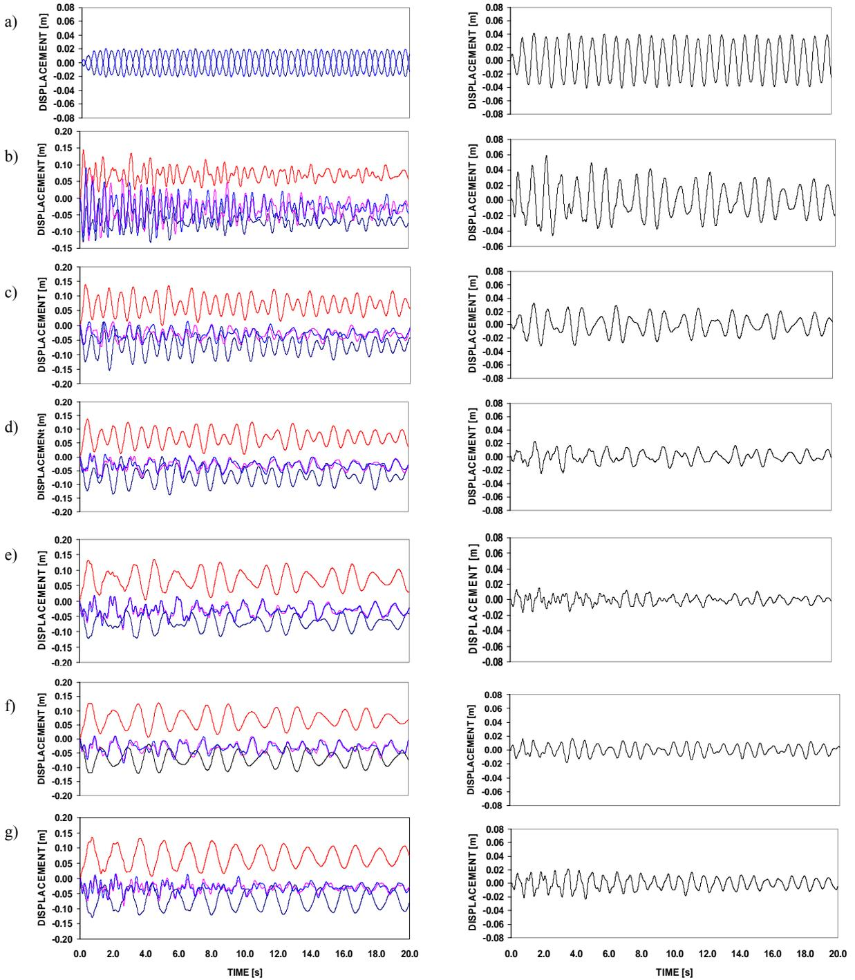
**Figure 2.** Displacement histories of two container nodes (dark blue and red) and two free surface nodes (light blue and magenta) (left column), and of liquid sloshing (right column). a) The rigid container, and flexible containers with added masses of b) 0 kg, c) 3 kg, d) 5 kg, e) 9 kg, f) 11 kg and g) 13 kg. Displacements are observed at the marked locations in Figure 1.
