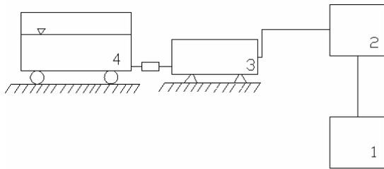
**Figure 5.** Schematic view of the experimental setup with base excitation. 1: personal computer, 2: power amplifier, 3: electromagnetic shaker, 4: container.
