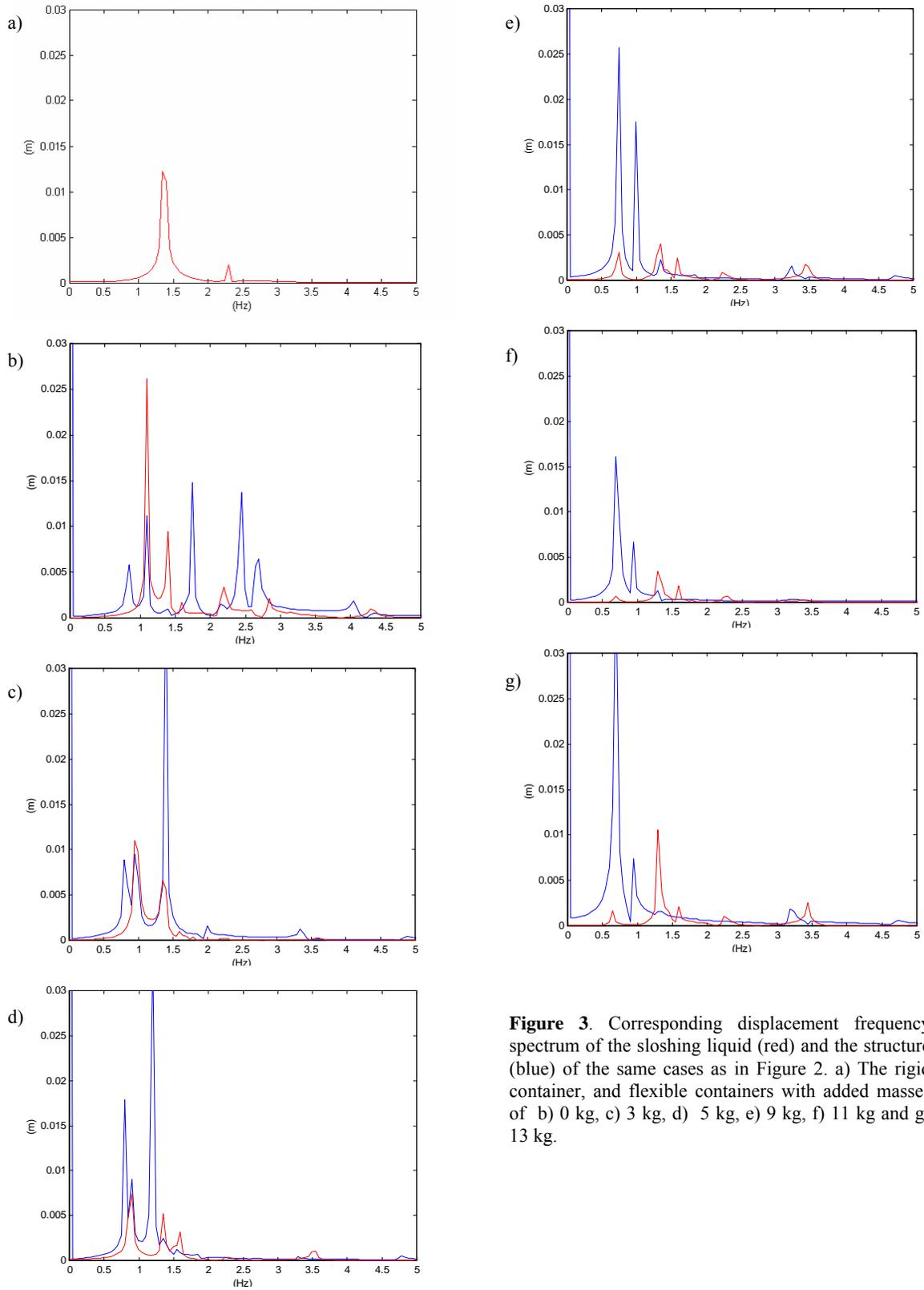
**Figure 3.** Corresponding displacement frequency spectrum of the sloshing liquid (red) and the structure (blue) of the same cases as in Figure 2. a) The rigid container, and flexible containers with added masses of b) 0 kg, c) 3 kg, d) 5 kg, e) 9 kg, f) 11 kg and g) 13 kg.
