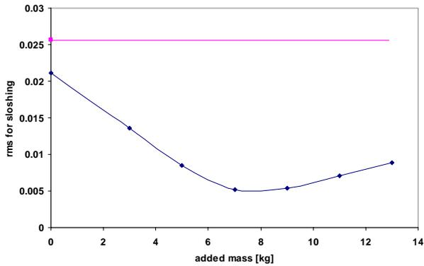
**Figure 4.** Variation of the rms sloshing magnitude in m with mass for rigid (—○—) and flexible (—■—) containers from numerical predictions.
