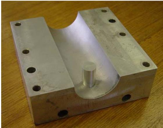
**Figure 4.** Photograph of flow geometry for erosion tests. Pipe inside diameter was 53mm. Arrow shows the flow direction.
