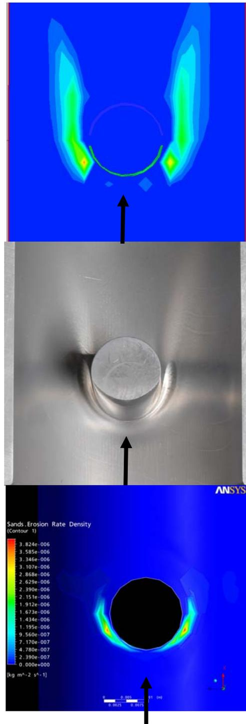
**Figure 10.** Top view of the erosion distribution in the cylinder and pipe flow. This shows clearly the effect of the horseshoe vortex. Top is measurement by CMM, middle is photograph of aluminium model after erosion and bottom is CFD prediction using the model of Grant and Tabakoff (1975) at the same scale as the measured erosion in the top figure. Arrows show flow direction.
