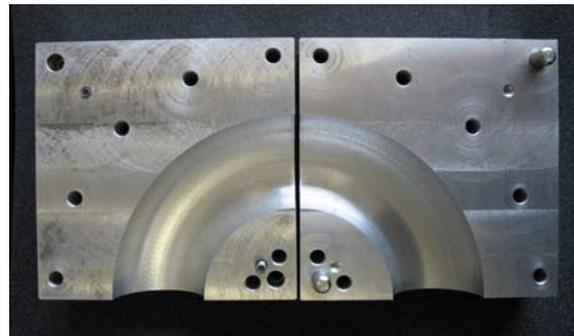
**Figure 2.** CNC machined aluminium elbow sections. This is a benchmark standard 1.5D elbow. Pipe diameter is 53mm.
