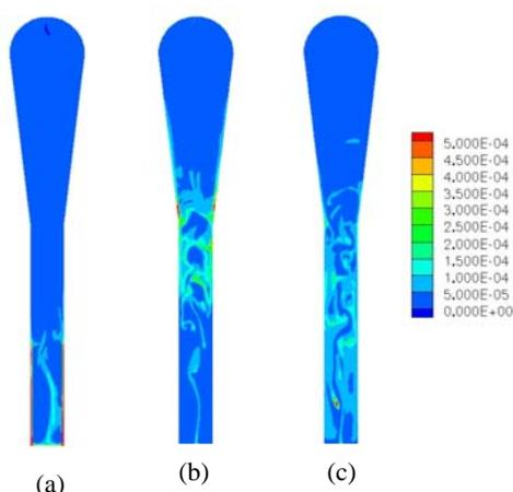
**Figure 7:** Instantaneous contours of catalyst with (a) negative charge, (b) positive charge and (c) zero charge.
