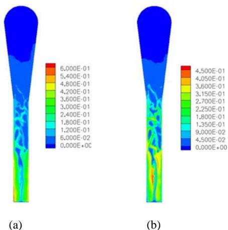
**Figure 4:** Instantaneous contours of solids volume fraction for (a) medium and (b) large particles with strong charges.
