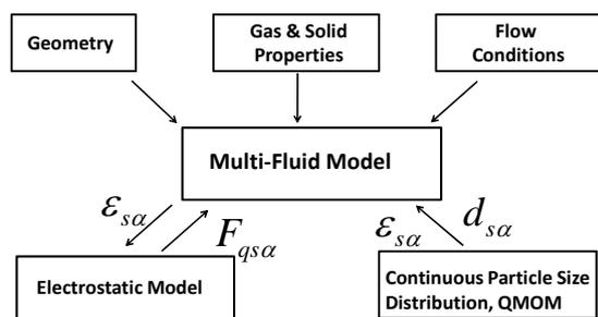
**Figure 1:** Coupling of electrostatic and multi-fluid CFD model.
