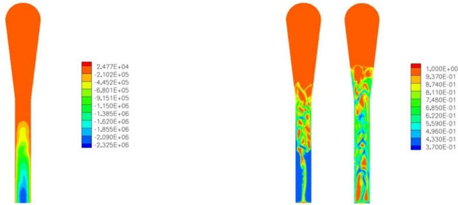
**Figure 3:** Instantaneous contours of electric potential (volts/m) with strongly charged particles.
