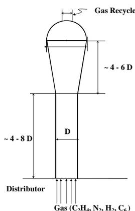
**Figure 2:** Sketch of pilot-plant fluidized-bed reactor.
