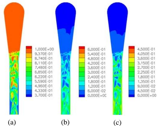
**Figure 6:** Instantaneous contours of volume fraction for (a) gas phase (b) medium particles, and (c) large particles with normal charges.
