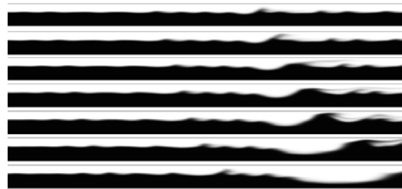
Figure 10: Calculated picture sequence at J_L = 1.0 m/s and J_G = 5.0 m/s (depicted part of the channel: 1.4 to 6 m after the inlet)
