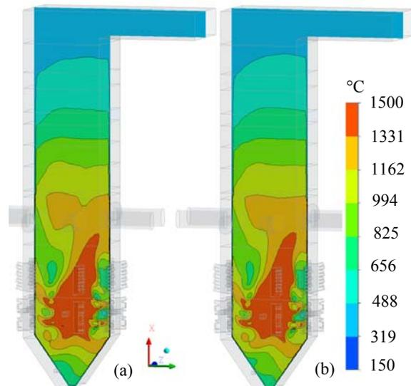
**Figure 7:** Predicted gas temperature profiles of mid-plane: (a) standard k- $\epsilon$  model, (b) SST model, case 2.
