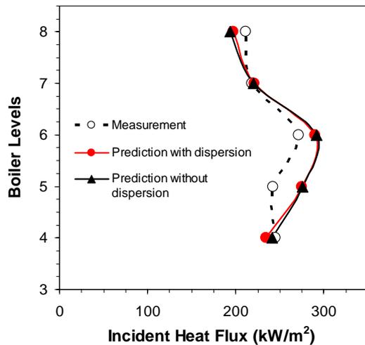
**Figure 6:** Comparison of calculated and measured wall incident heat flux profiles, burner 4&6 off at MCR. (Measurements from HRL, 2005)
