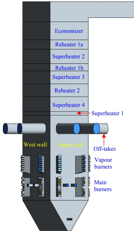
**Figure 1:** CFD geometry of Yallourn W unit No. 3
