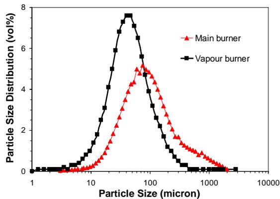
Figure 2: Mill coal particle size distribution at main and vapour burners.
