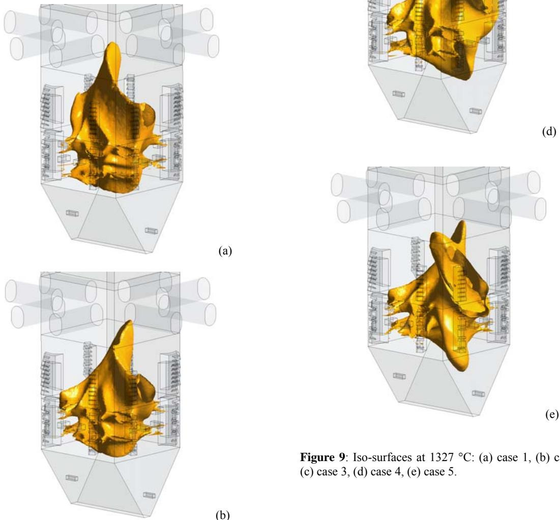
**Figure 9:** Iso-surfaces at 1327 °C: (a) case 1, (b) case 2, (c) case 3, (d) case 4, (e) case 5.
