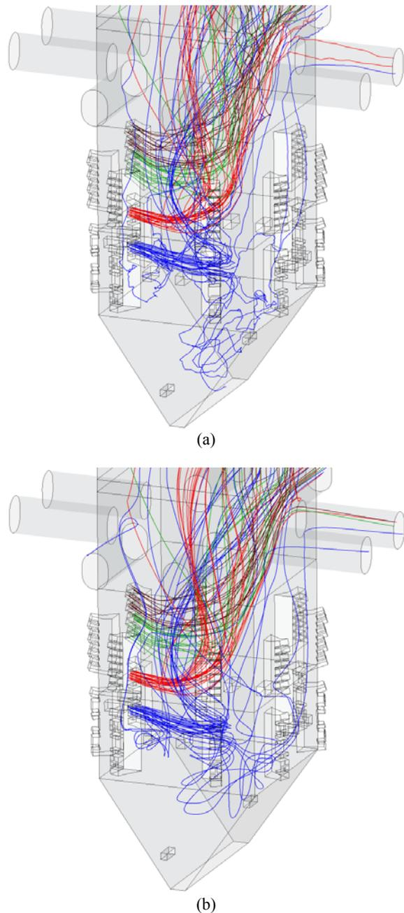
**Figure 8:** Predicted particle trajectories of case 3: (a) with particle dispersion, (b) without particle dispersion.
