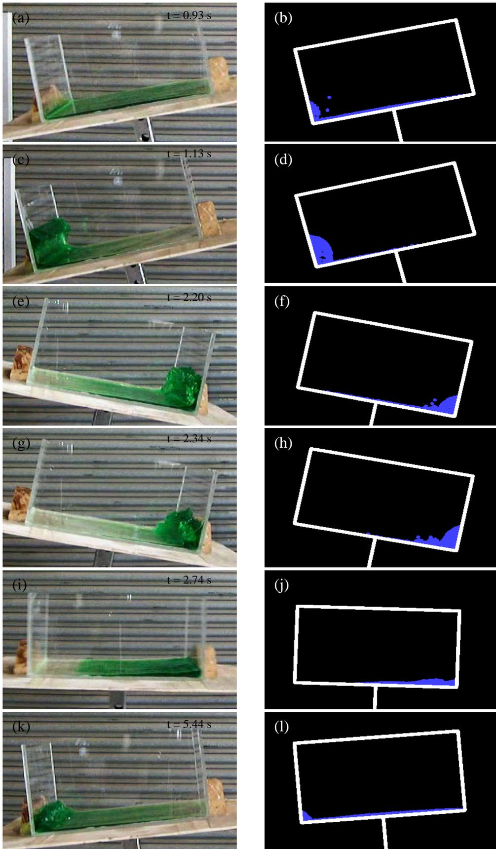
**Figure 3:** Free surface comparisons of 5.5 mm liquid depth at different marked instances. Left column has the experimental observations and right column has the numerical predictions.
