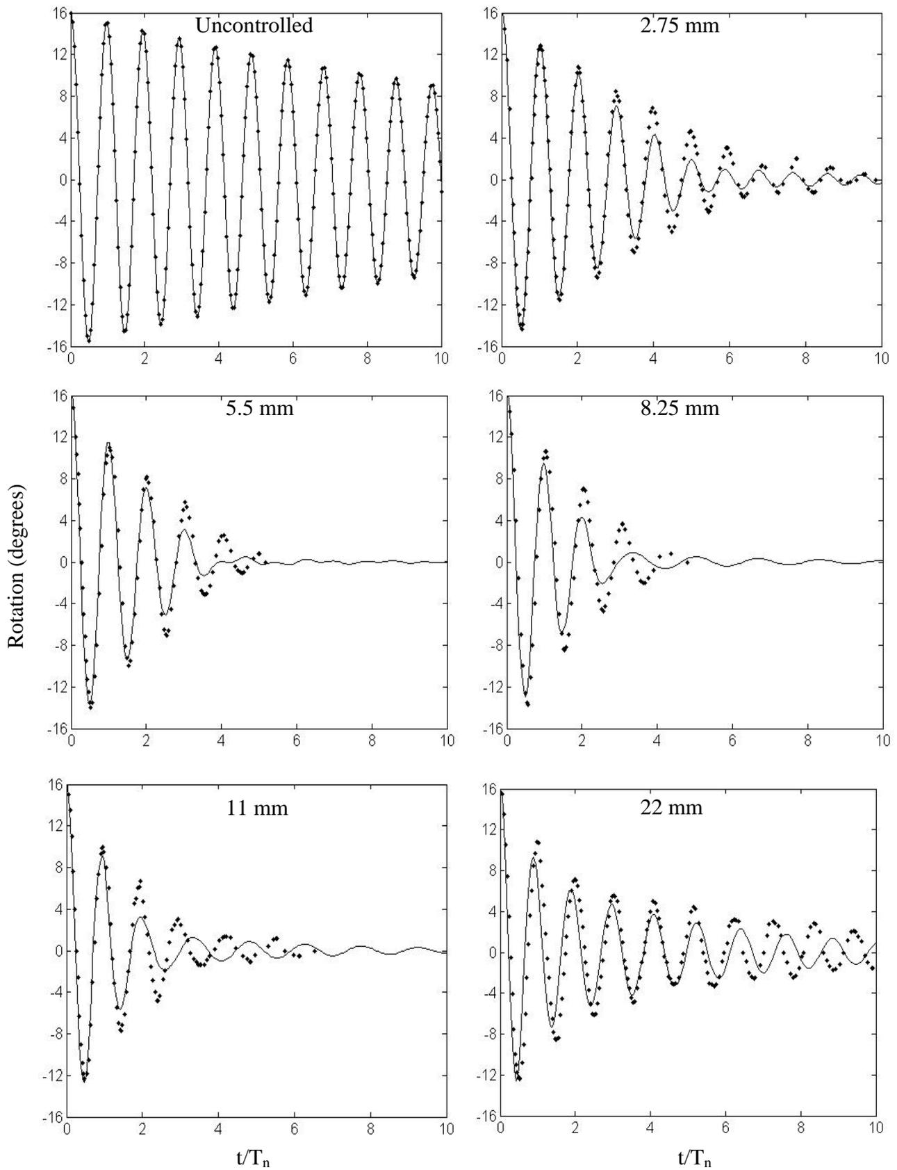
**Figure 5:** History of angular displacement of experimental observations (●) and SPH predictions (—) for (a) uncontrolled, (b) 2.75 mm, (c) 5.5 mm, (d) 8.25 mm, (e) 11 mm and (f) 22 mm deep cases.
