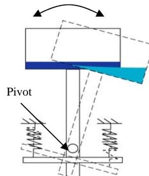
**Figure 2:** Showing the structure and the sloshing absorber at rest (vertical) and at initially displaced positions.
