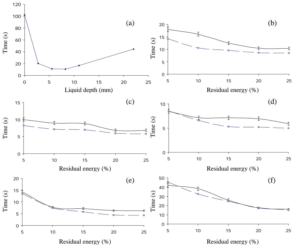
**Figure 4:** (a) Variation of experimentally observed settling time with liquid depths and comparisons for (b) 2.75 mm, (c) 5.5 mm, (d) 8.25 mm, (e) 11 mm and (f) 22 mm liquid depths between experiments (—) and predictions (---).
