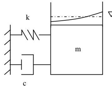
**Figure 1:** Tuned liquid damper, attached to a mechanical oscillator of mass  $m$ , stiffness  $k$  and viscous damping coefficient of  $c$ .
