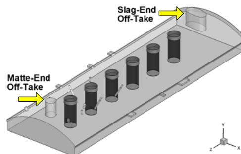
**Figure 2:** The freeboard CFD model geometry.
