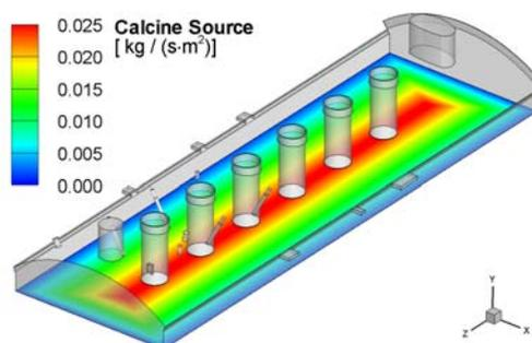
**Figure 3:** The prescribed distribution of gas flow from the calcine.
