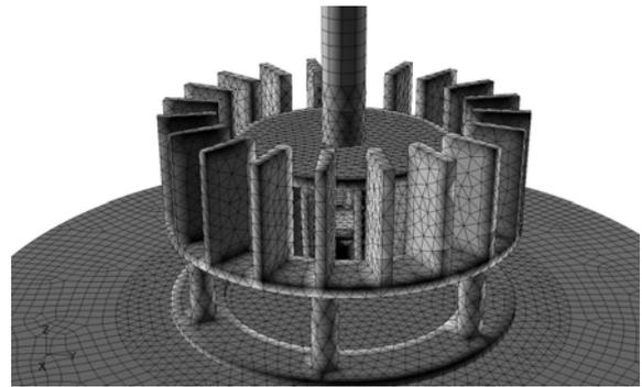
**Figure 4:** The structured-unstructured computational mesh on the 102 mm Outotec FloatForce rotor-stator system.
