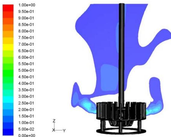
**Figure 6:** The region in the flotation cell where the critical bubble pressure (0.28 Pa) is exceeded ( $p_b^+$  in Pa).
