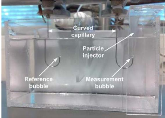
**Figure 2:** Bubble pressure experiment (bubble diameter 1 mm).
