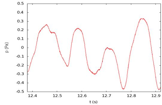
**Figure 3:** Bubble pressure versus time during bubble-particle collision and attachment ( $d_b = 1$  mm,  $d_p = 150\text{-}180$   $\mu\text{m}$ , quartz).
