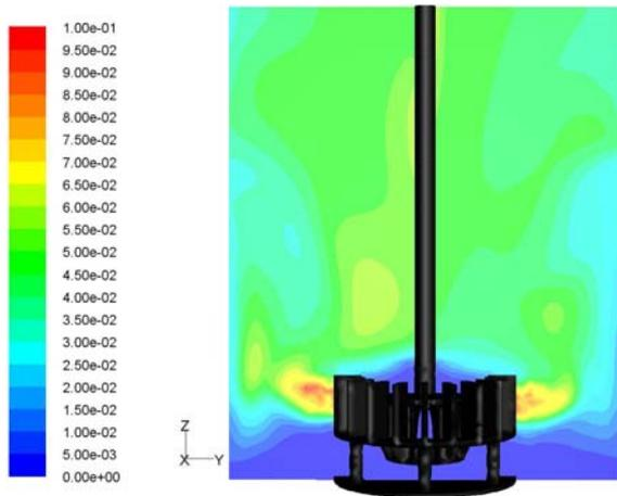
**Figure 5:** CFD simulation result for volume fraction of air in the Outotec flotation cell.
