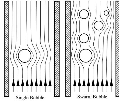
**Figure 1:** Profile of liquid velocity passing through single bubble and multi-bubbles
