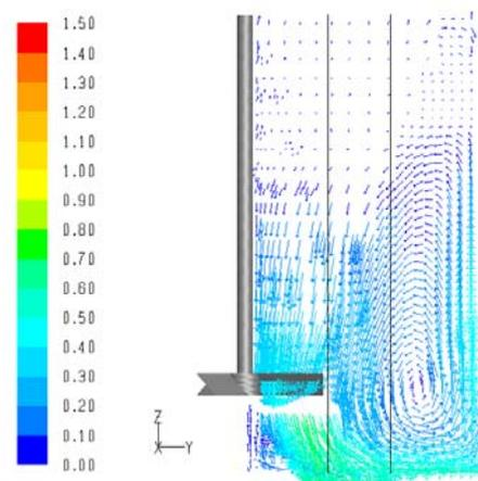
**Figure 3:** Instantaneous particle velocity vectors (m/s) calculated with mixture model. Radial measurement locations  $r=105$  mm and  $r=185$  mm are marked with vertical lines. 5% solid volume fraction.
