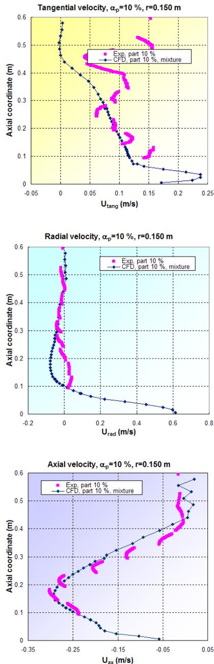
**Figure 10:** Time-averaged particle velocity components on radial location  $r=150$  mm. 10% solid volume fraction.
