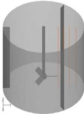
**Figure 2:** Geometry of the mixing tank. The radial measurement locations are illustrated with orange vertical lines.
