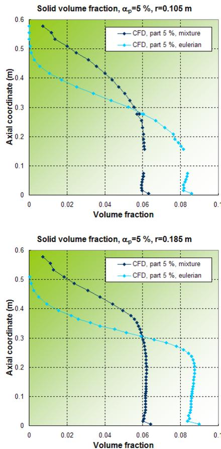
**Figure 7:** Time-averaged particle volume fractions on radial locations  $r=105$  mm and  $r=185$  mm. 5% solid volume fraction.
