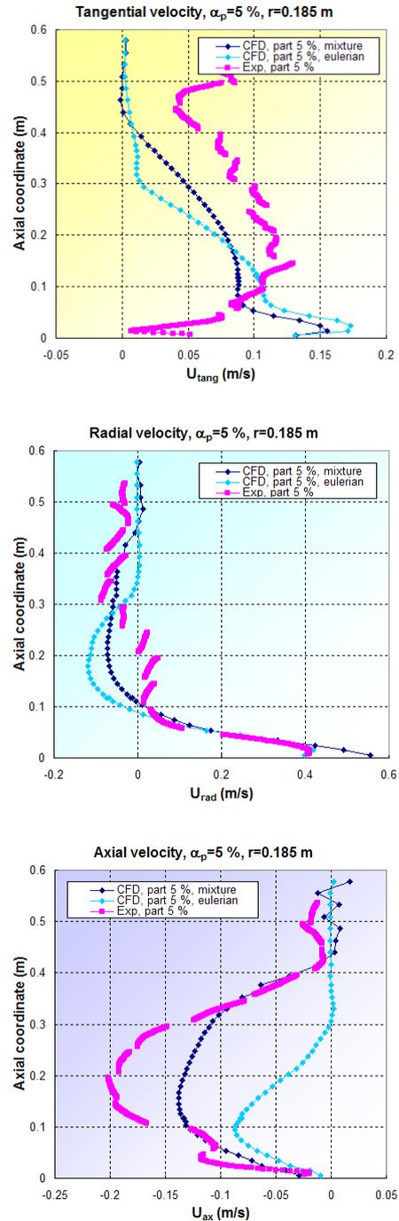
**Figure 9:** Time-averaged particle velocity components on radial location  $r=185$  mm. 5% solid volume fraction.
