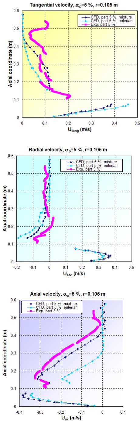
**Figure 8:** Time-averaged particle velocity components on radial location  $r=105$  mm. 5% solid volume fraction.
