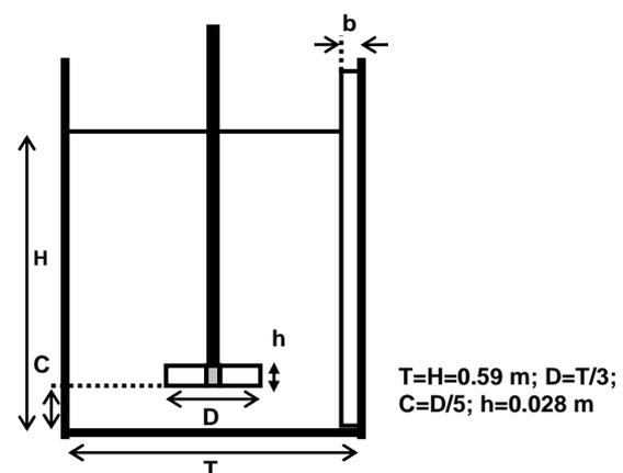
**Figure 1:** Schematic diagram of the tank geometry.
