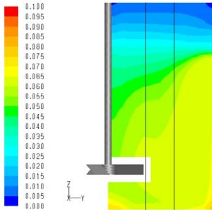
**Figure 4:** Time-averaged solid volume fraction calculated with mixture model. 5% solid volume fraction.
