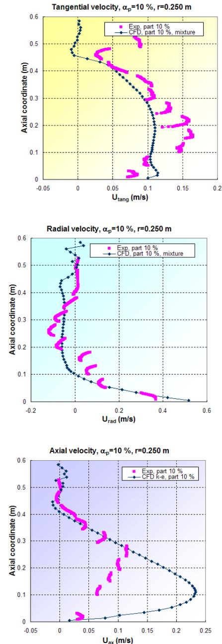
**Figure 11:** Time-averaged particle velocity components on radial location  $r=250$  mm. 10% solid volume fraction.
