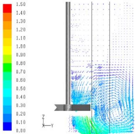
**Figure 5:** Instantaneous particle velocity vectors (m/s) calculated with Eulerian model. Radial measurement locations  $r=105$  mm and  $r=185$  mm are marked with vertical lines. 5% solid volume fraction.
