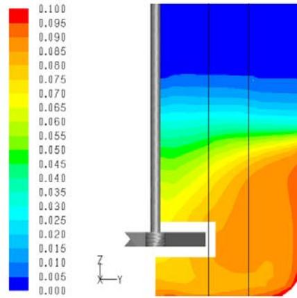
**Figure 6:** Time-averaged solid volume fraction calculated with Eulerian model. 5% solid volume fraction.
