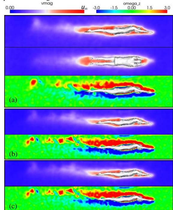
**Figure 4:** Instantaneous speed and span-wise vorticity of the towed male swimmer in different cross-sections for, (a)  $u_\infty = 1.0$  m/s, (b)  $u_\infty = 1.5$  m/s, and (c)  $u_\infty = 2.0$  m/s.
