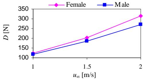
**Figure 5:** Towing drag force versus speed at 0.5 m depth.
