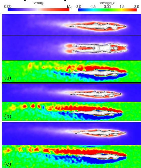
**Figure 3:** Instantaneous speed and span-wise vorticity of the towed female swimmer in different cross-sections for, (a)  $u_\infty = 1.0$  m/s, (b)  $u_\infty = 1.5$  m/s, and (c)  $u_\infty = 2.0$  m/s.
