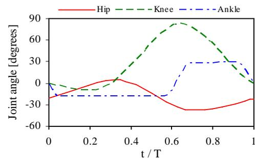
**Figure 8:** Leg joint angles throughout the dolphin kick swimming cycle. Angles are with respect to the initial pose given in Figure 6.
