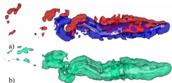
**Figure 13:** Instantaneous isosurfaces in the fluid around the swimmer performing dolphin kick at  $t = 1.37$  s for case B. (a)  $\omega_z = 3$  is red and  $\omega_z = -3$  is blue, and (b)  $|\omega| = 5$ .
