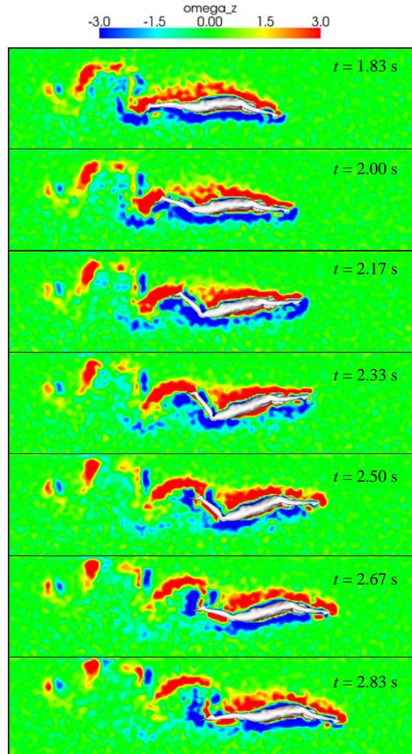
**Figure 11:** Instantaneous span-wise vorticity contours ( $\omega_z$ ) on the  $z = 0$  (sagittal) plane throughout a single dolphin kick cycle for case A.
