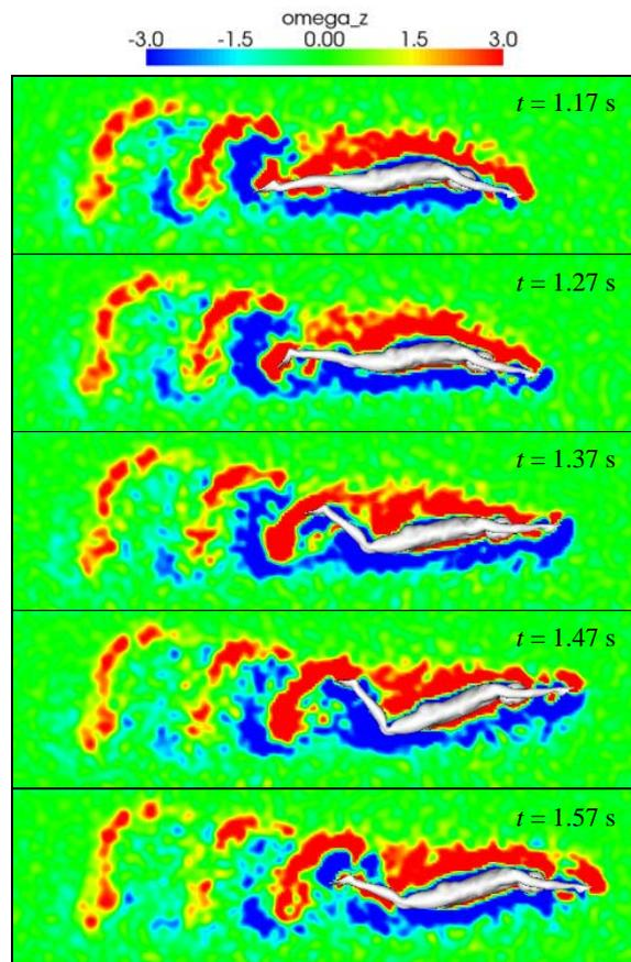
**Figure 12:** Instantaneous span-wise vorticity contours ( $\omega_z$ ) on the  $z = 0$  (sagittal) plane throughout a single dolphin kick cycle for case B.
