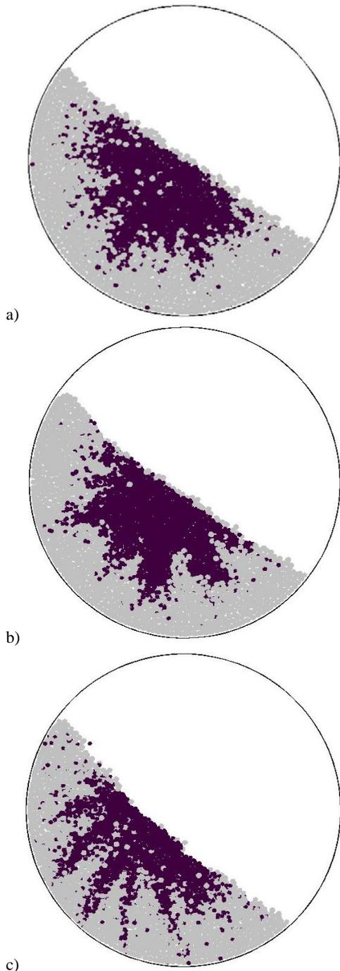
**Figure 5:** Snap-shots of simulations with super-quadric particles for various values of  $n$ . (a)  $n = 2.2$ , (b)  $n = 2.5$  and (c)  $n = 3.0$ . All other parameters are exactly the same for all three simulations.
