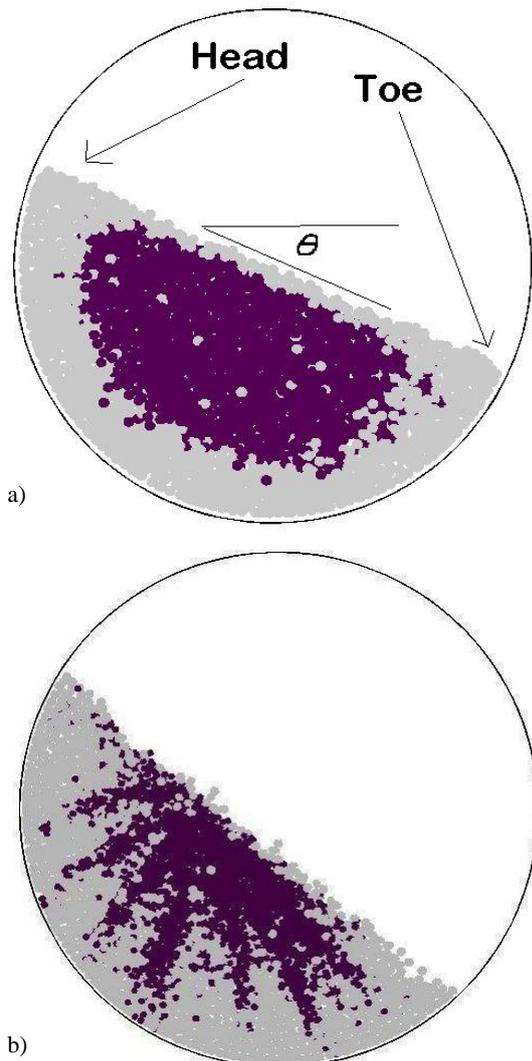
**Figure 1:** Comparison of stable, equilibrium particle distribution for (a) a periodic slice, and (b) short cylinder. The smaller, denser particles are dark grey while the larger, less dense particles are light grey. The cylinder rotates clockwise. In (a) the slope angle of the top surface is labelled ( $\theta$ ), which is equal to the angle of repose. The “head” and “toe” of the bed are also marked.
