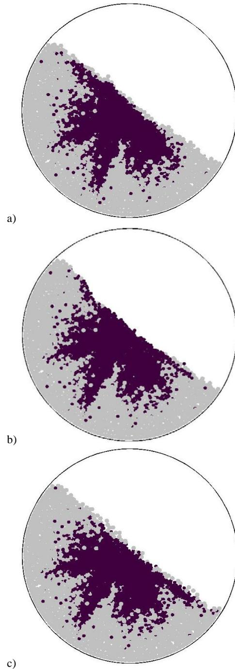
**Figure 2:** Changes in shape of top surface during streak formation. (a) At  $t=500s$  the interface is initially flat with slope angle equal to angle of repose. (b) At  $t=502s$  the slope of free surface increases in region near head of bed. (c) At  $t=503s$  the angle of failure is exceeded and the surface near the head collapses with particles avalanching down the free surface. The streak now appears at toe of bed.
