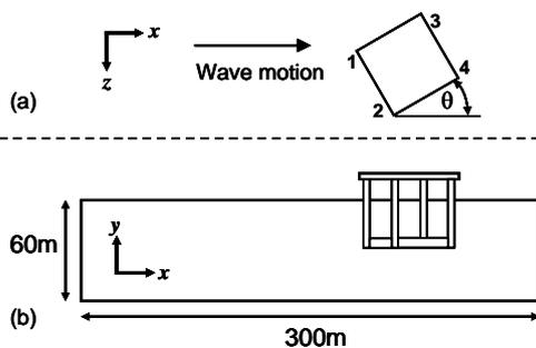
Figure 2: Computational domain. (a) plan view ( $x$ - $z$  plane) showing orientation with respect to the wave motion ( $\theta$ ) and 1-4 denote mooring cable ID. (b) elevation view ( $x$ - $y$  plane). Domain size is  $x=300$  m,  $z=150$  m.
