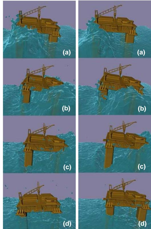
**Figure 6:** Side view of 8-LS (left) and TLP (right) platforms for normal ( $0^\circ$ ) wave impact. From top to bottom times are 8, 10, 12 and 16 s.
