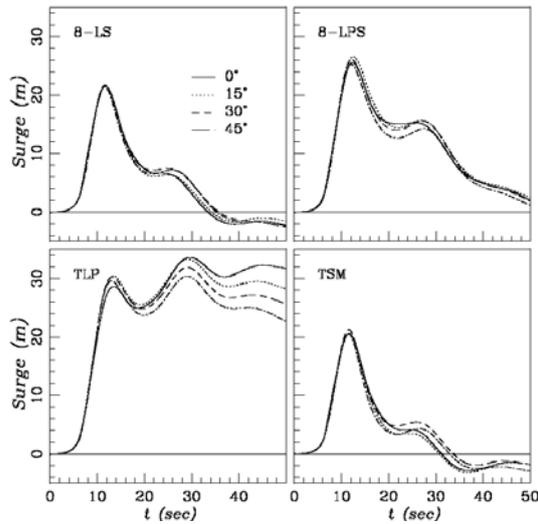
**Figure 7:** Surge response for the different mooring systems at 4 different wave impact angles.
