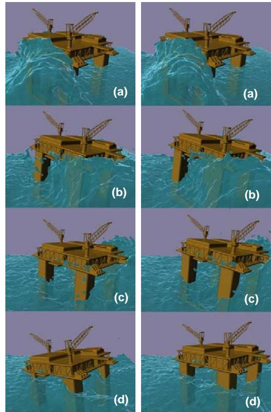
**Figure 9:** Side view of 8-LS (left) and TLP (right) platforms for a 45° wave impact. From top to bottom times are 8, 10, 12 and 16 s.
