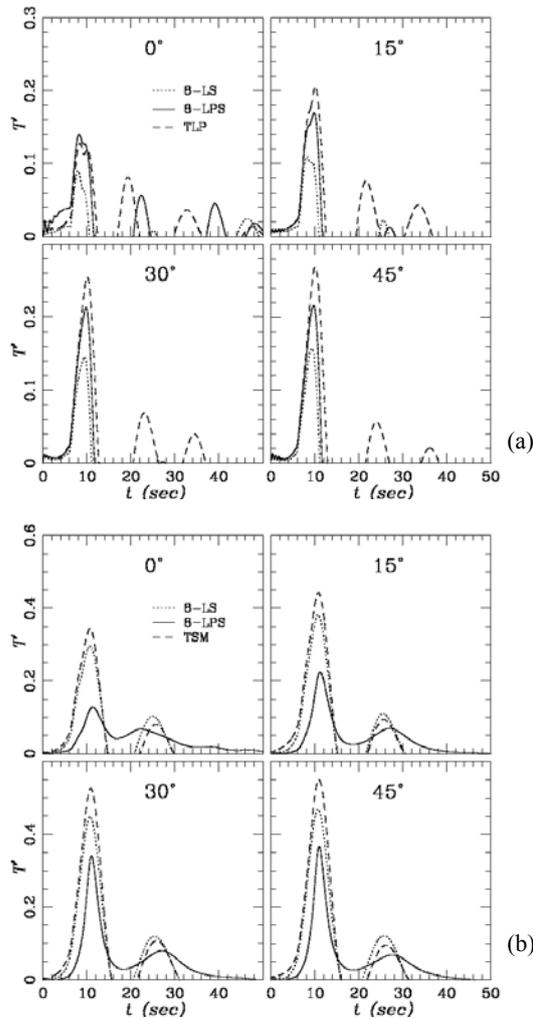
**Figure 10:** Cable tension in leading edge (a) vertical mooring cables and (b) diagonal cables. Tension has been normalised by the platform weight.
