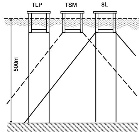
Figure 3: Schematic of the mooring systems. Left is the Tension Leg (TLP) system, centre is the Taut Spread Mooring system (TSM) and right is a combination of both (or "8L", 8 lines system). The diagonal cables make an angle of 45 degrees with the ocean floor.
