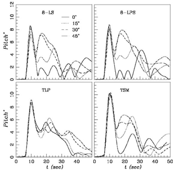
**Figure 5:** Pitch response for different wave impact angles for the 4 different mooring systems.
