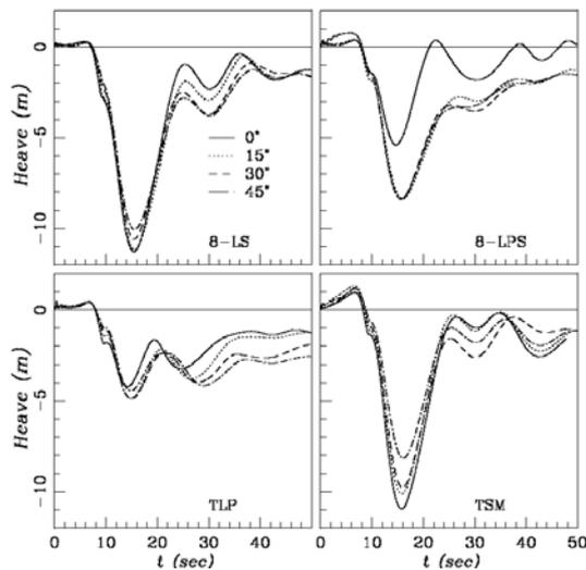
**Figure 8:** Heave response for different mooring systems at 4 different wave impact angles.
