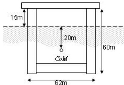
Figure 1: Schematic of the semi-submersible platform.
