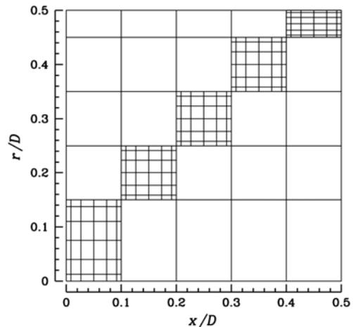
**Figure 2:** An example of a spectral element mesh in the meridional semi-plane for the cylindrical-coordinate formulation used here. Internal node points are drawn in selected elements for a tensor-product polynomial shape function order  $N=6$ . The axial domain length corresponds to an axial wavenumber  $\alpha = 2\pi/0.5 = 12.57$ .
