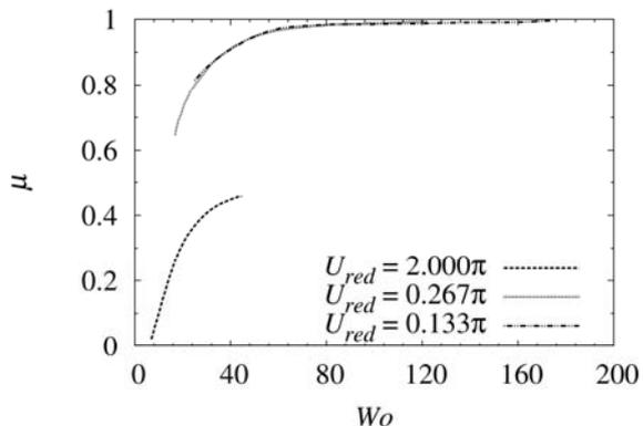
**Figure 4.** Yang & Yih (1977) dominant Floquet multiplier data for axisymmetric modes ( $k = 0$ ) with  $\alpha = 4$ . Note that here (as opposed to Figure 3) there is no collapse with Womersley number.
