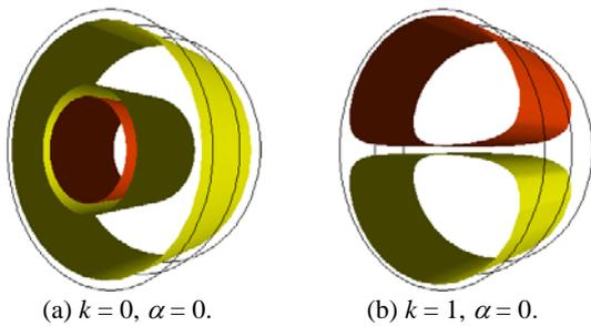
**Figure 7** Comparison of (a) axisymmetric ( $k = 0$ ) and (b) non-axisymmetric ( $k = 1$ ) Floquet mode shapes, both axially invariant,  $\alpha = 0$ . Visualized as isosurfaces of positive/negative axial velocity component. Computed at  $Wo = 97$ .
