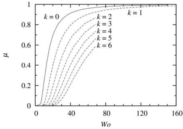
**Figure 6** Dominant Floquet multipliers for axially invariant modes,  $\alpha = 0$ , both axisymmetric ( $k = 0$ ) and non-axisymmetric ( $k > 0$ ) as functions of Womersley number.
