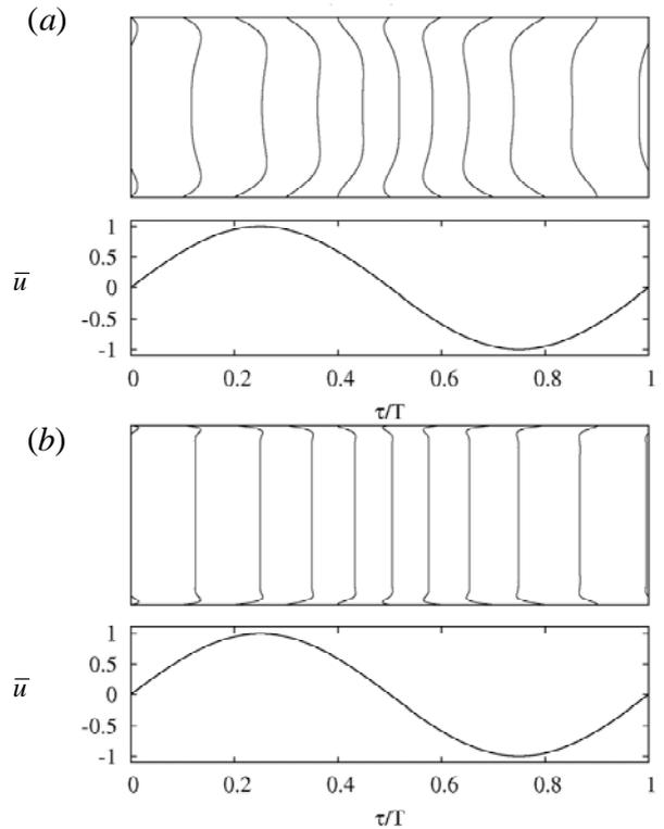
**Figure 1:** Shows radial velocity profiles at different base-flow phases – note the reversed flow lags in the near-wall region by up to  $90^\circ$ . The area-average flow speed  $\bar{u}(t)$  is shown as a function of time for oscillatory base flows with (a)  $Wo=10.23$ ; (b)  $Wo=35.5$ .
