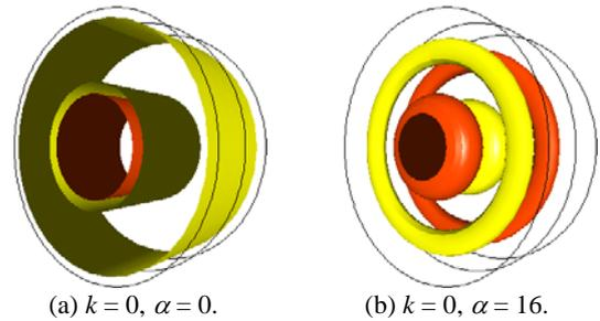
**Figure 5** Comparison of axisymmetric ( $k = 0$ ) Floquet mode shapes; (a) axially invariant,  $\alpha = 0$ ; (b) with axial wavenumber  $\alpha = 16$ . Visualized as isosurfaces of positive/negative axial velocity component.
