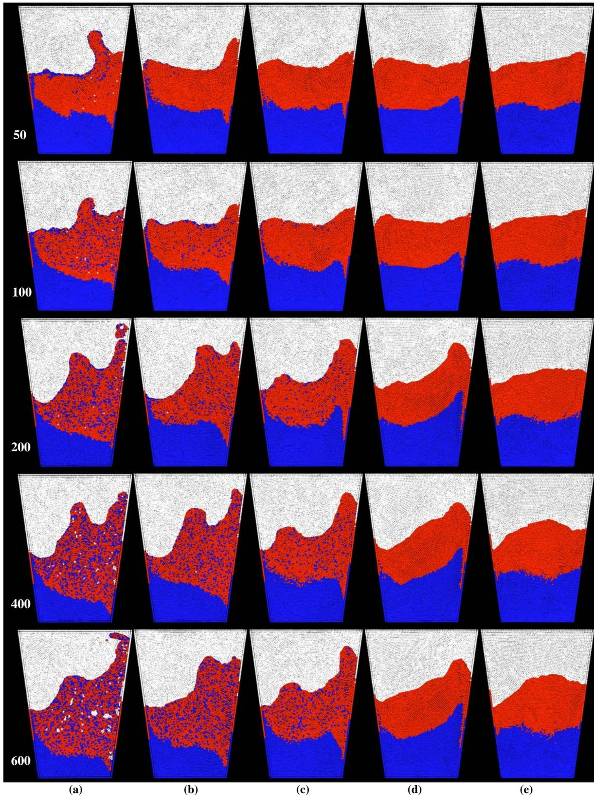
**Figure 3:** Mixing between two liquids, with density ratio  $\rho_L/\rho_H =$  (a) 1.0 (b) 0.9 (c) 0.8 (d) 0.7 and (e) 0.1. The heavier liquid ( $\rho_H$ ) is coloured blue and the lighter liquid ( $\rho_L$ ) is coloured red. The air pocket at the top is coloured white. The rows represent duration of mixing non-dimensionalised by the shaker rotation cycle time. The mixing pattern is compared at 50, 100, 200, 400 and 600 cycles.
