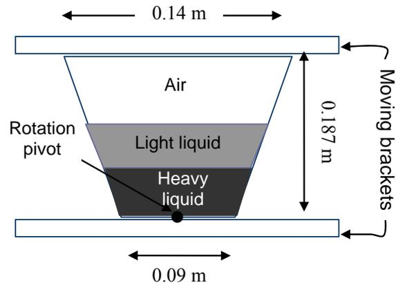
**Figure 1:** Schematic of the shaker used for viscous liquid mixing.
