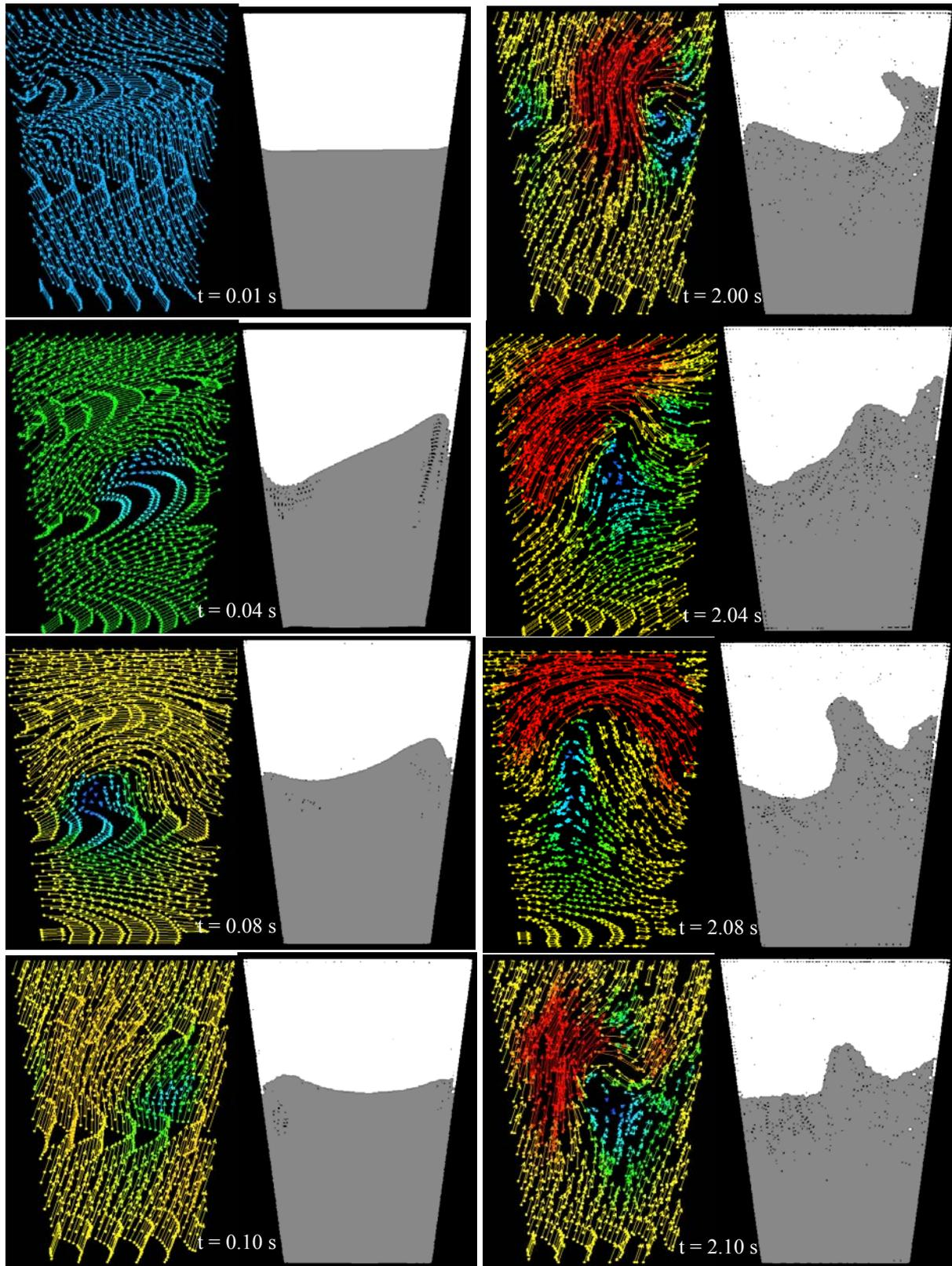
**Figure 2:** Flow and mixing pattern in the shaker for a 50% viscous liquid fill level and  $\rho_l/\rho_H = 1.0$ . At each time there is a pair of pictures with the fluid coloured by velocity on the left and by its material type on the right. For velocity colouring, blue indicates 0.0 m/s and red indicates 1.5 m/s. The white fluid is air whereas the grey coloured fluid is the viscous liquid. It takes 0.1 s for one shaker cycle. A periodic flow pattern develops after 2.0 s.
