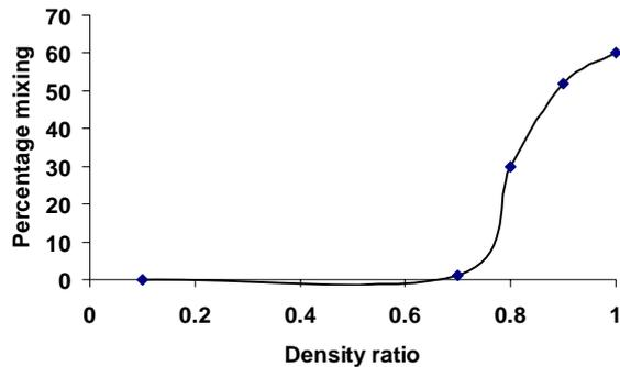
**Figure 5:** Change in percentage mixing with density ratio between the lighter and heavier liquid after the mixing has reached its asymptotic limit.
