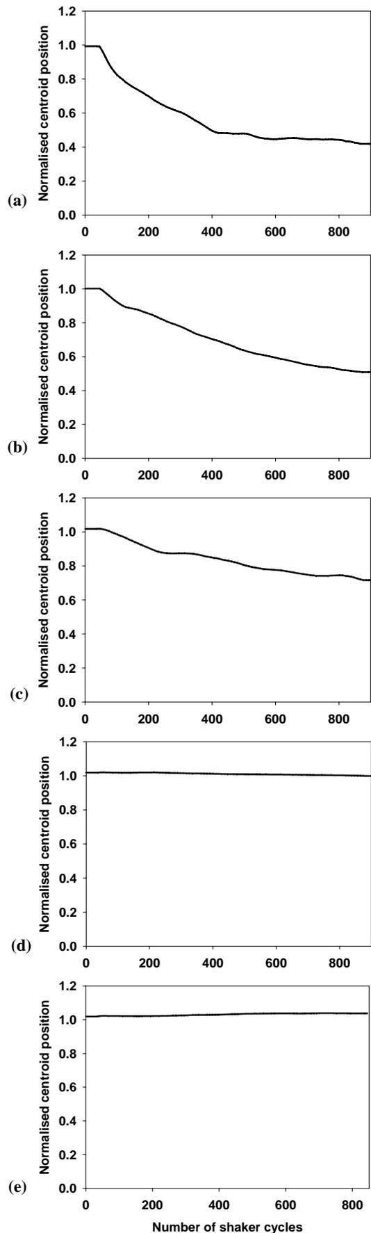
**Figure 4:** Change in centroid position with shaker rotation cycle for  $\rho_H/\rho_L =$  (a) 1.0 (b) 0.9 (c) 0.8 (d) 0.7 and (e) 0.1.
