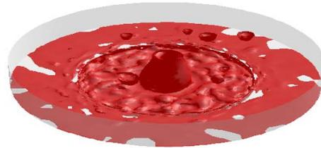
**Figure 2:** Computed volume fraction of water for 2D (a) and 3D (b) model.  $Q = 18 \text{ ml s}^{-1}$ ,  $\omega = 21 \text{ Rad sec}^{-1}$ , 2D radius 15 cm, 3D radius 3.5 cm.
