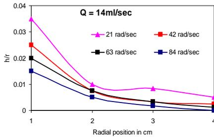
**Figure 4:** Effect of rotational speed on the non dimensional liquid film thickness  $Q = 14 \text{ ml s}^{-1}$ , Disc diameter = 10 cm.
