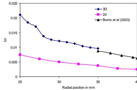
**Figure 6:** Effect of volumetric flow rate on measured and calculated non dimensional film thickness.  $Q = 10 \text{ ml s}^{-1} \omega = 21 \text{ Rad sec}^{-1}$ , 2D radius 15 cm, 3D radius 3.5 cm.
