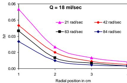
**Figure 5:** Effect of rotational speed on the non dimensional liquid film thickness  $Q = 18 \text{ ml s}^{-1}$ , Disc diameter = 10 cm.
