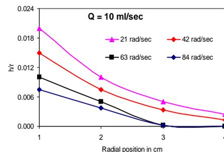
**Figure 3:** Effect of rotational speed on the non dimensional liquid film thickness  $Q = 10 \text{ ml s}^{-1}$ , Disc diameter = 10 cm
