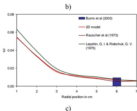
**Figure 7:** Non dimensional film thickness on a 10cm diameter disc for varying volumetric flow rate.
