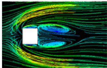
**Figure 9:** Comparison of streamlines in symmetry plane (left)  $z/H=0$  and (right) first cell from bottoms' wall.  $Re_H=40,000$ .
