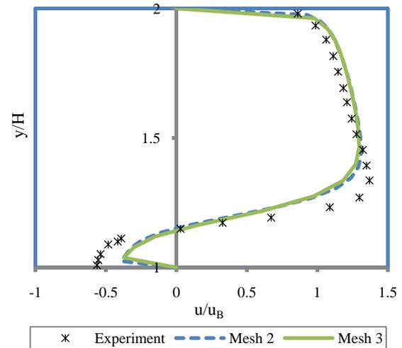
**Figure 7:** Comparison of mean streamwise velocity profiles in the symmetry line  $x/H=0.5$  using RSM, at  $Re_H=40,000$ .
