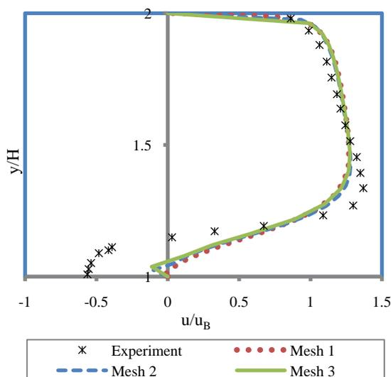
**Figure 6:** Comparison of mean streamwise velocity profiles in the symmetry line  $x/H=0.5$  using Standard  $k-\varepsilon$ , at  $Re = 40,000$ .
