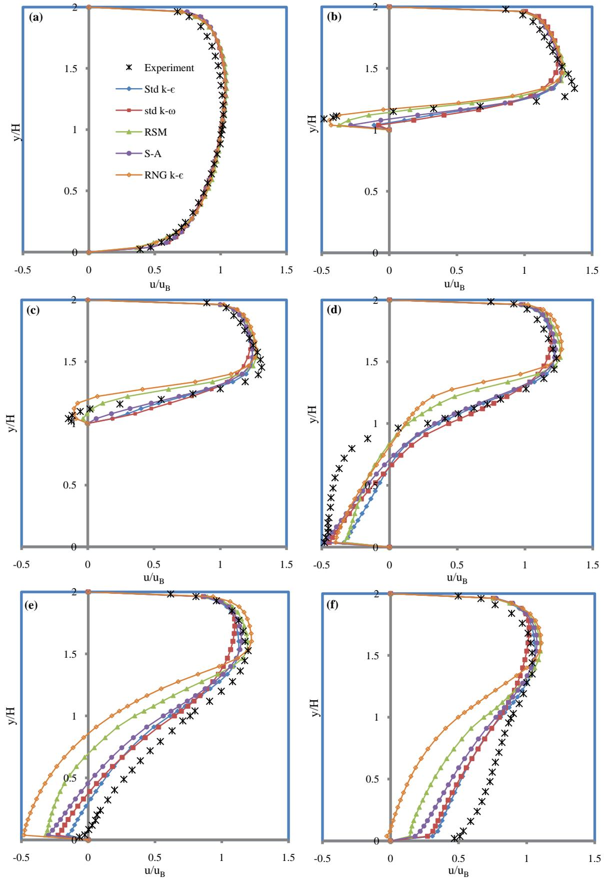
**Figure 8:** Comparison of the mean streamwise velocity profiles of Mesh 3 in the symmetry line (a)  $x/H=-1.0$ , (b)  $x/H=0.5$  (c)  $x/H=1.0$ , (d)  $x/H=1.5$ , (e)  $x/H=2.5$  and (f)  $x/H=4.0$ , for  $Re_H = 40,000$ . Legends are the same in all plots.
