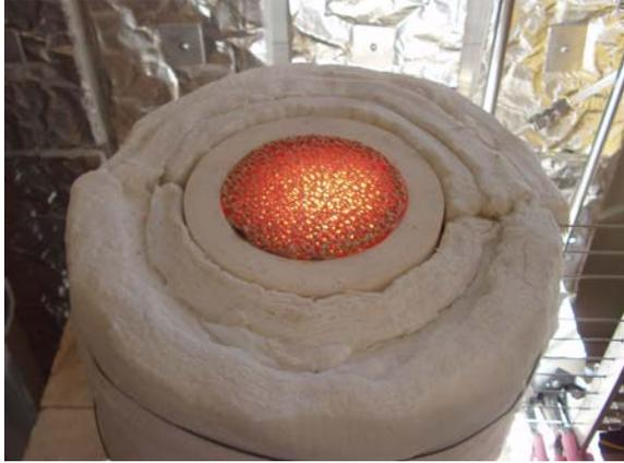
**Figure 1:** The heated surface of a porous burner.
