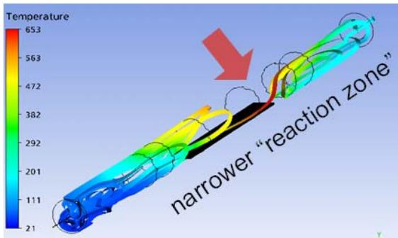
**Figure 13** Flow streamlines through a point in the reaction zone predicted using CFD model. (Argon carrier gas flow of 1L/min and all heater temperatures 705°C.)
