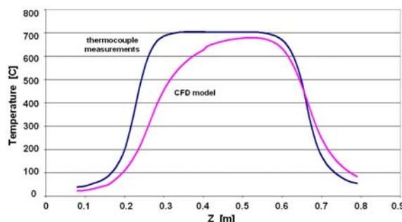
**Figure 4** Temperature measured using bare thermocouple on reactor centre line compared with CFD prediction. (Helium carrier gas flow of 1L/min and all heater temperatures 705°C.)
