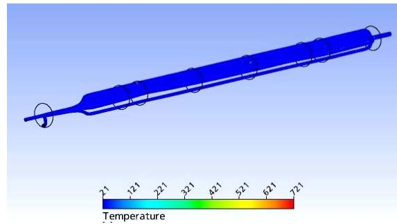
**Figure 8** Flow streamlines in reactor at ambient temperature predicted using CFD model. (Helium carrier gas flow of 1L/min.)
