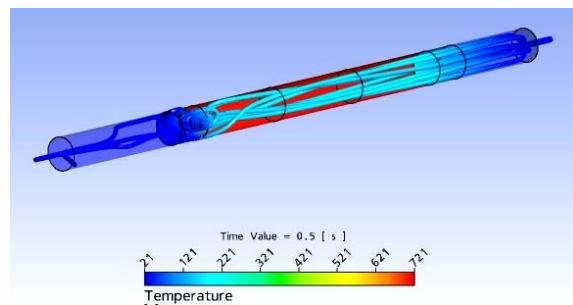
**Figure 9** Swirling flow near the reactor inlet is predicted to develop around 0.5 seconds after all heaters reach operating temperature. (Helium carrier gas flow of 1L/min and all heater temperatures 705°C.)
