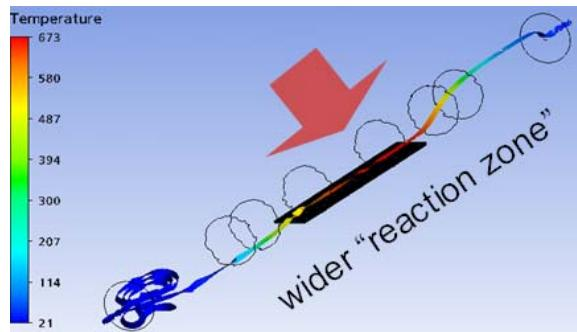
**Figure 11** Flow streamlines through a point in the reaction zone predicted using CFD model. (Helium carrier gas flow of 1L/min and all heater temperatures 705°C.)
