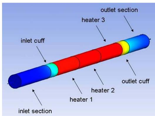
**Figure 6** Schematic of CFD model of tube furnace
