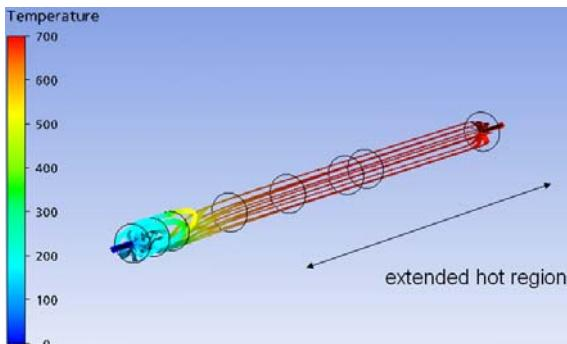
**Figure 15** Flow streamlines in reactor with shortened inlet section and insulated outlet section predicted using CFD model. (Helium carrier gas flow of 1L/min and all heater temperatures 705°C.)
