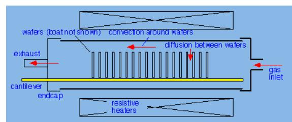
Figure 2 Schematic of commercial tube furnace for processing wafers for use in electronics industry (Timedomain CVD, Inc., 2009).
