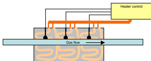
Figure 1 Schematic of tube furnace reactor
