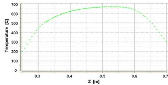
**Figure 12** Temperature profile along the flow streamlines through a point in the reaction zone predicted using CFD model. (Helium carrier gas flow of 1L/min and all heater temperatures 705°C.)
