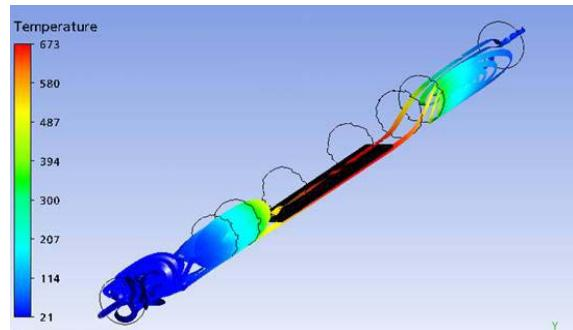
**Figure 7** Flow streamlines in reactor predicted using CFD model. (Helium carrier gas flow of 1L/min and all heater temperatures 705°C.)
