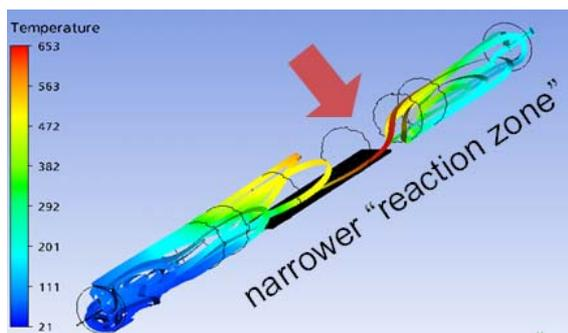
**Figure 13** Flow streamlines through a point in the reaction zone predicted using CFD model. (Argon carrier gas flow of 1L/min and all heater temperatures 705°C.)
