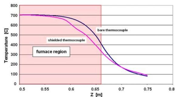
**Figure 5** Temperature measurements in exit end of reactor. (Helium carrier gas flow of 1L/min and all heater temperatures 705°C.)
