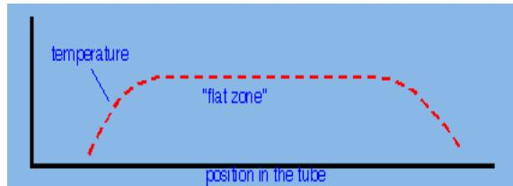
**Figure 3** Temperature profile in commercial tube furnace (Timedomain CVD, Inc., 2009).
