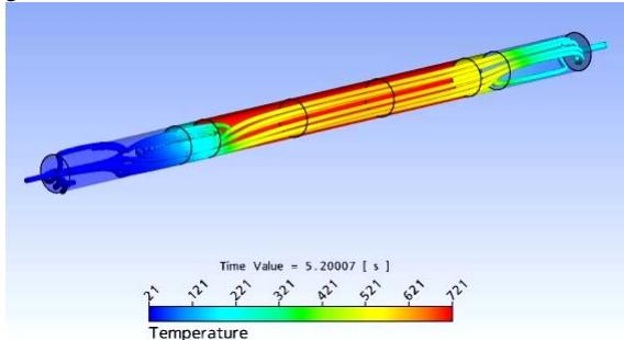
**Figure 10** Swirling flow near the reactor outlet is predicted to develop around 5.2 seconds after all heaters reach operating temperature. (Helium carrier gas flow of 1L/min and all heater temperatures 705°C.)
