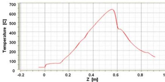
**Figure 14** Temperature profile along the flow streamlines through a point in the reaction zone predicted using CFD model. (Argon carrier gas flow of 1L/min and all heater temperatures 705°C.)
