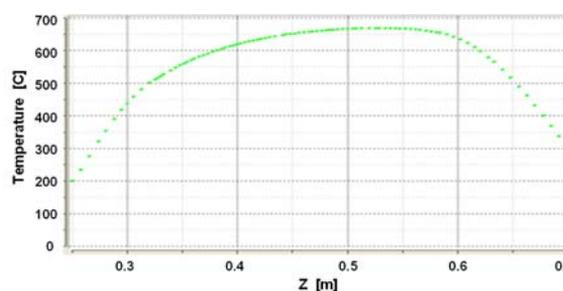
**Figure 12** Temperature profile along the flow streamlines through a point in the reaction zone predicted using CFD model. (Helium carrier gas flow of 1L/min and all heater temperatures 705°C.)
