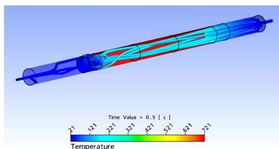
**Figure 9** Swirling flow near the reactor inlet is predicted to develop around 0.5 seconds after all heaters reach operating temperature. (Helium carrier gas flow of 1L/min and all heater temperatures 705°C.)
