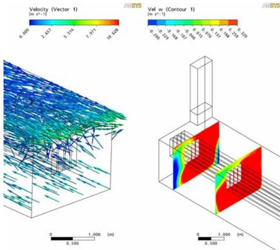
**Figure 8:** Left vector plot of velocities in the tunnel. Right close up of velocities in between and around the bars. Note positive w velocity is from the inlet to the stack.
