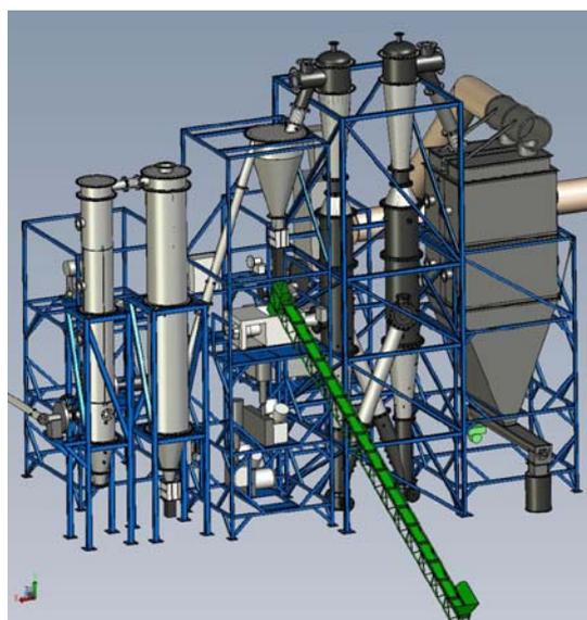
**Fig.1** UC Discovery/West Biofuels 5 ton/day dual-fluidized bed reactor based on the “Pyrox” design at the West Biofuels, Woodland Biomass Research Centre in Woodland, CA
