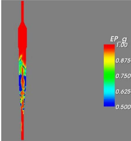
**Fig. 3.** A vertical section snapshot of dynamic simulation of the full gasifier column at steady state. (Table 2, Set A:  $d_p / D = .00639$ ,  $e=.85$ ) The colour scheme for gas void fraction  $EP\_g$  gives void fraction in the bed.
