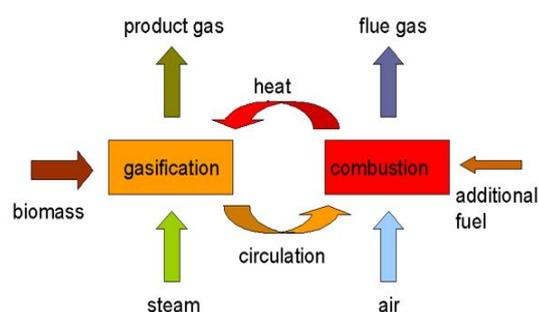
**Fig.2** Pyrox design Schematics.
