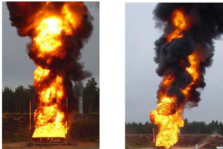
Figure 2: Instantaneous photographic images of TBPB \left(\frac{\bar{H}}{d} = 9\right) and TBPEH \left(\frac{\bar{H}}{d} = 8\right) pool fires ( d = 3.4 m)
