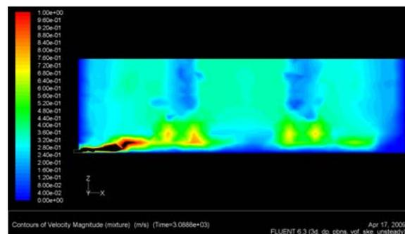
**Figure 10:** Velocity contours of reaction gasses in the charge materials during the tapping process
