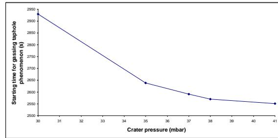
**Figure 8:** Relation between crater pressure and starting time of gassing taphole phenomenon.
