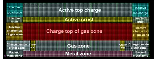
**Figure 3:** 2D view of different zones inside the silicon production furnace.
