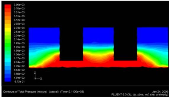
**Figure 5:** Pressure patterns inside the submerged arc furnace.
