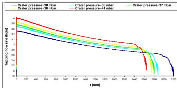
**Figure 6:** The effect of crater gas pressure on both the tapping flow rate and starting time of gassing taphole phenomenon.
