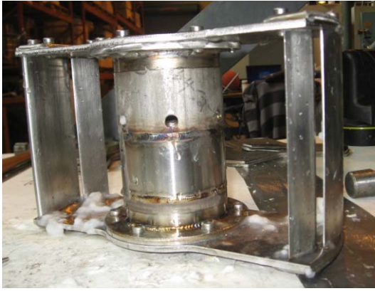
Figure 8: Photograph of prototype adjustable MEF rotor used in the pilot trials showing the slot between main foil and flap.
