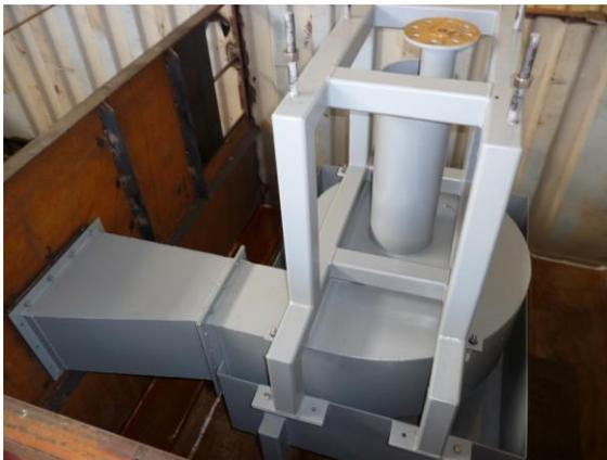
**Figure 7:** View of the inside of the test tank. The Turbodil pumps from one compartment to the other, returning via the adjustable gate in the central divider.
