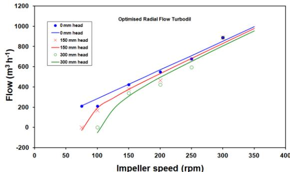
**Figure 12:** Flow vs. impeller speed for the radial Turbodil. Lines are the CFD predictions, dots are the measured values.
