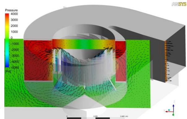
**Figure 5:** Flow and pressure fields of the radial flow option.
