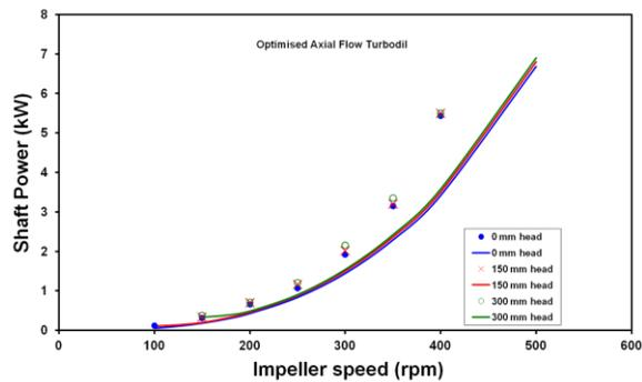
**Figure 11:** Power vs. impeller speed for the axial flow Turbodil. Lines are the CFD predictions, dots are the measured values. Note CFD is just the power to turn the impeller, whereas the measured values include losses from the motor and chain drive.
