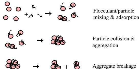
**Figure 1:** Flocculation process
