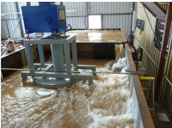
**Figure 8:** Radial flow impeller at 250 rpm with 0.3 m head.
