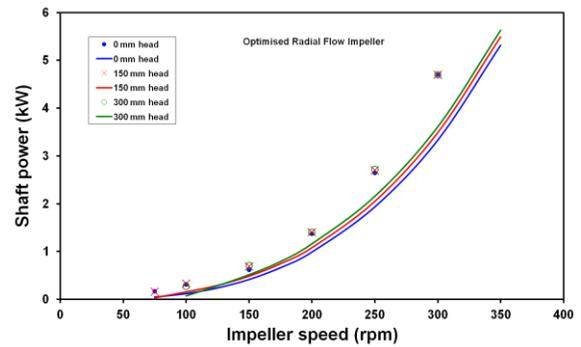
**Figure 13:** Power vs. impeller speed for the radial flow Turbodil. Lines are the CFD predictions, dots are the measured values.
