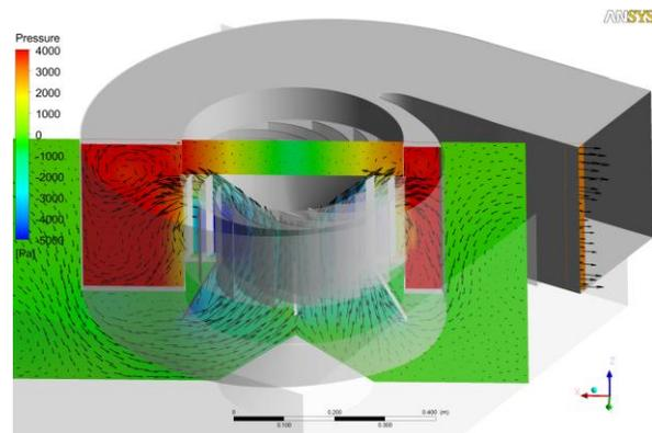
**Figure 5:** Flow and pressure fields of the radial flow option.
