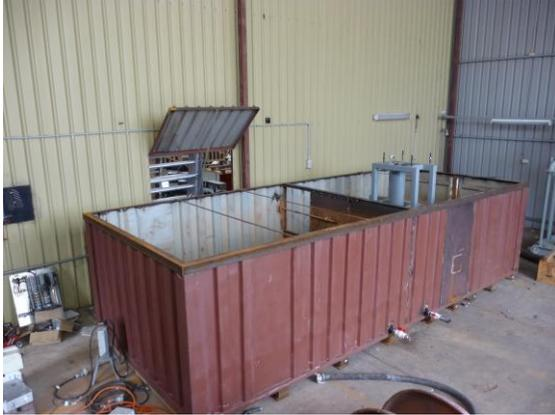
**Figure 6:** Test tank built from modified shipping container.
