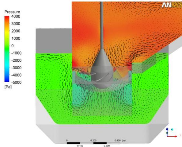
**Figure 4:** Flow and pressure fields of the axial flow option.
