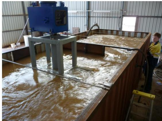
**Figure 9:** Radial flow impeller at 250 rpm ~0 m head.
