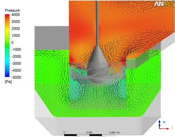
**Figure 4:** Flow and pressure fields of the axial flow option.
