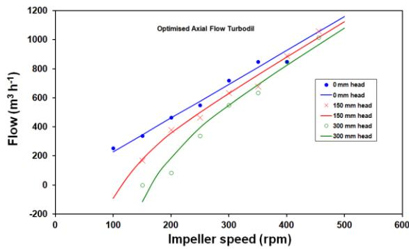
**Figure 10:** Flow vs. impeller speed for the axial flow Turbodil. Lines are the CFD predictions, dots are the measured values.
