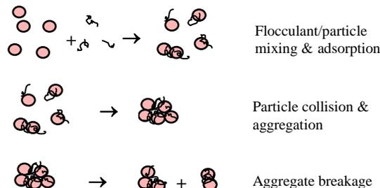
**Figure 1:** Flocculation process
