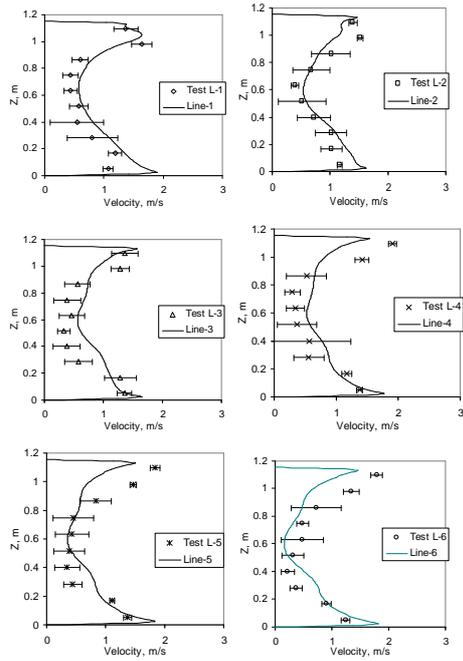
**Figure 7:** Comparison of velocity profiles at Plane-1 (for case with three perforated plates and collection plates)
