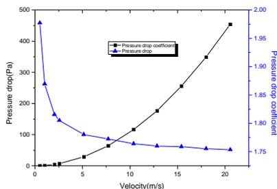
**Figure 12:** Overall pressure drop character through the ESP unit with different velocity
