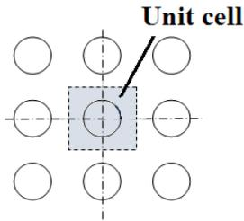
Figure 2: Unit cell definition.
