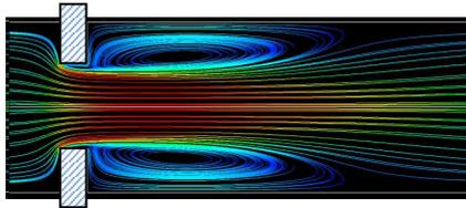
Figure 3: Flow stream line through a unit cell orifice
