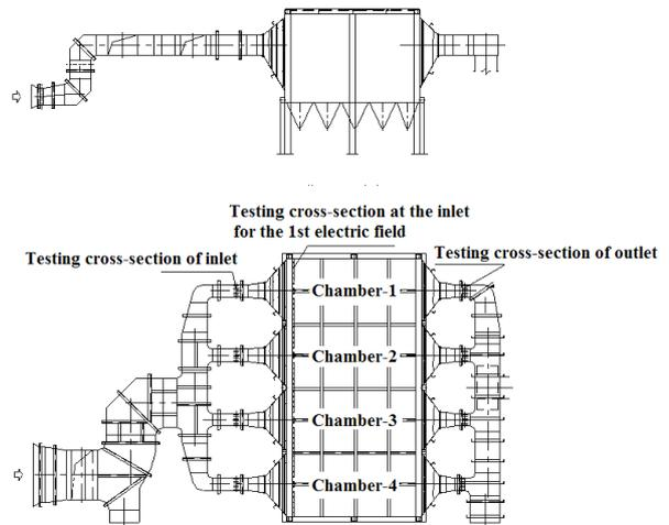
**Figure 9:** The schematic drawing of the general layout
