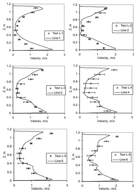
**Figure 8:** Comparison of velocity profiles in Plane-2 (for case with three perforated plates)
