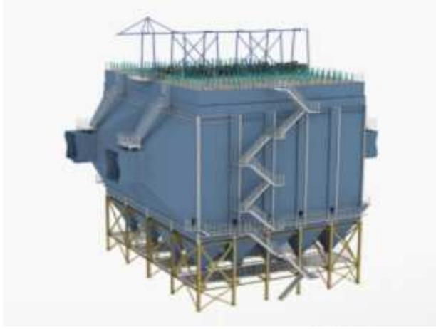
**Figure 1:** Typical structure of ESP
