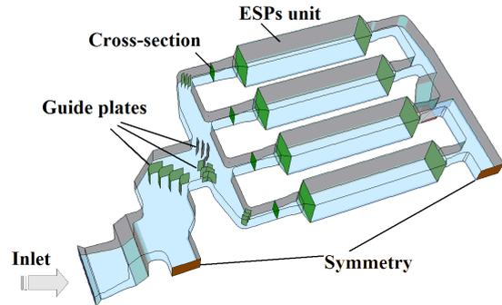
**Figure 13:** Configuration of whole system for flow distribution simulation
