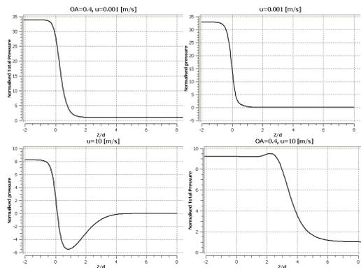
Figure 4: Streamwise distribution of pressure along the centreline for different inlet velocities ( $f=0.4$ ).
