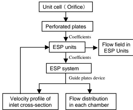
**Figure 10:** Simulation procedure of ESP system
