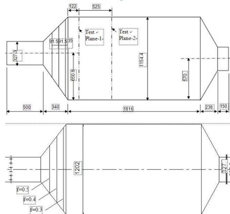
Figure 5: Base ESP chamber model and dimensions
