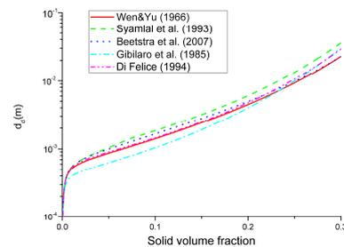
Figure 1. Cluster diameter predicted by EMMS model with different microscopic drag correlations
