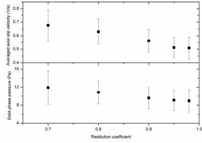
Figure 3. Comparison of averaged axial slip velocity and solid phase pressure obtained from different restitution coefficients.  $\bar{\mathcal{E}}_s = 0.05$ .
