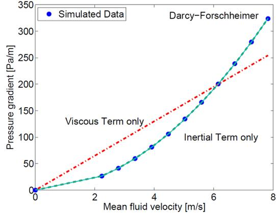
**Figure 2:** Pressure Drop  $v$  Mean velocity. Blue dots represent the simulated data (same as Table 1). The curves represent the three fitting options: Darcy law, Viscous or Inertial term only.
