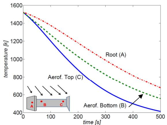
**Figure 6:** Cooling curve prediction for different locations inside the turbine blade.
