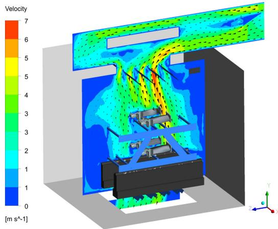
**Figure 7:** Velocity magnitude in a furnace loaded with 6 blades. Full scale model where every component is explicitly modelled.
