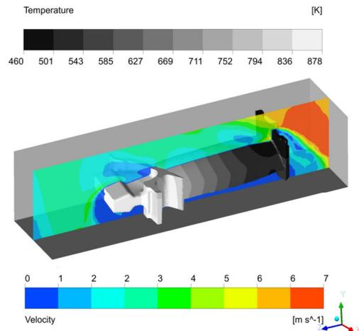
**Figure 5:** Detailed flow field around a turbine blade, modelled individually (micro scale model) and associated temperature distribution on the surface.
