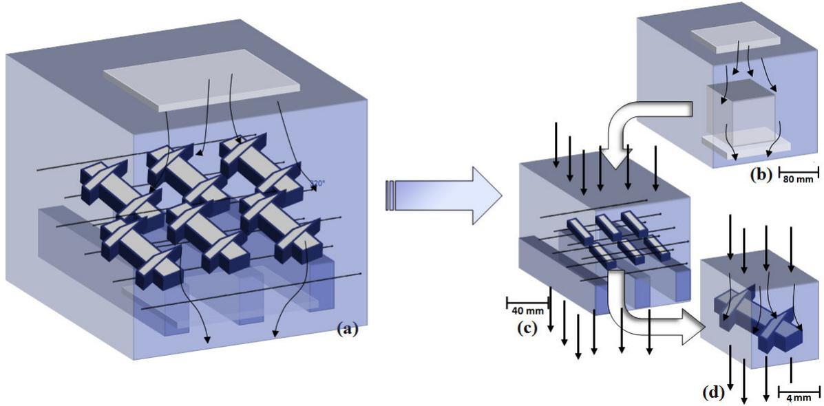
**Figure 1:** Schematic illustration of the multi level decomposition of the laboratory scale vacuum furnace used in this study.
