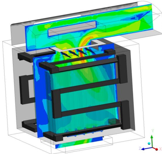
**Figure 3:** Velocity magnitude field on an x-cut of the macro model of the furnace. The fixtures like rack and support, as well as the specimen are missing, replaced by a porous medium.
