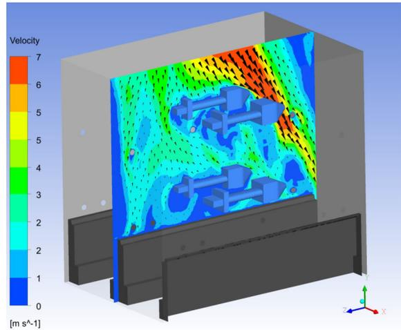
**Figure 4:** X-cut plane that shows velocity magnitude field within the furnace load. In the meso scale model the load is made up of blades with a simplified shape.
