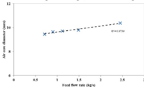
**Figure 6:** Numerical predictions of air core for different feed flow rates.
