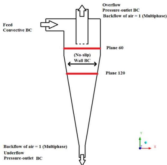
**Figure 1:** Schematic illustration of the boundary conditions.
