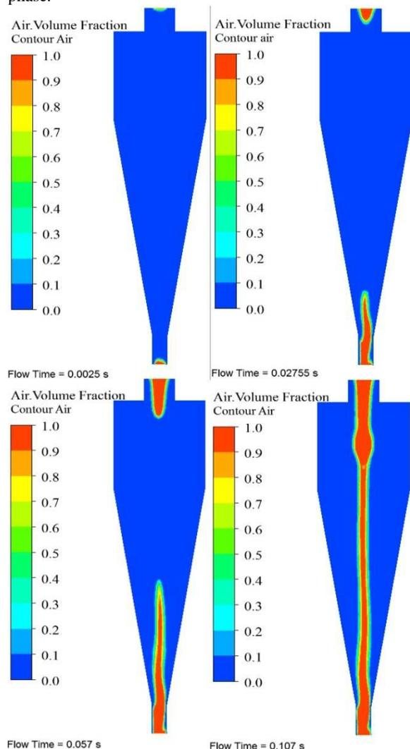
**Figure 4:** Air core development process.
