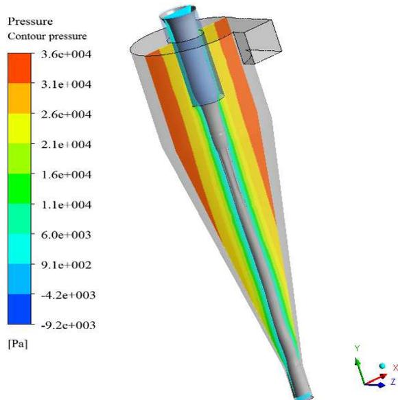
**Figure 3:** Pressure contour plot and the developed air core based on the single-phase modelling
