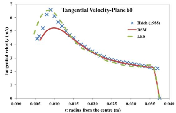
**Figure 2:** Comparison of two different turbulence models for prediction of tangential velocity in Plane 60.
